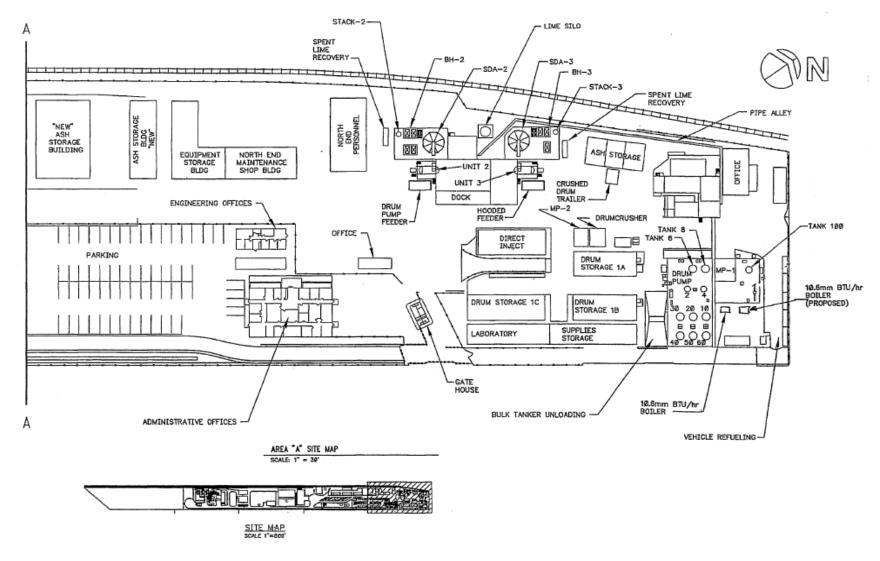
Figure 1. Layout of Veolia's Facility Showing Units 2 and 3.
