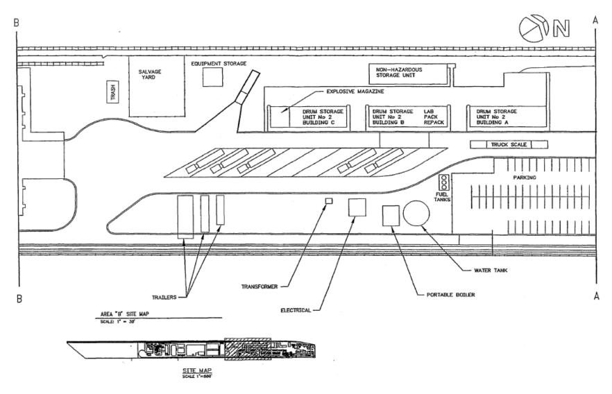
Figure 2. Layout of Veolia's Facility Showing Drum Storage and Lab Pack Repack Areas.
