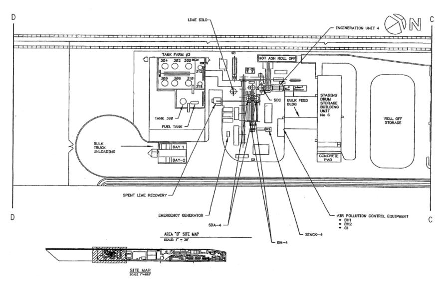
Figure 4. Layout of Veolia's Facility Showing Incineration Unit 4 and Associated Emission Units.
