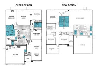
kitchen, bathrooms, and laundry areas—as close as possible to the hot water heater. By designing our homes with kitchens and baths concentrated in one area of the house, we vastly reduce the length and complexity of the required plumbing runs. The example on the bottom left demonstrates what a difference centralized plumbing can make. In the older KB Home design, plumbing is located in five different areas of the house, while the new design only requires two.
