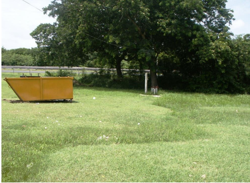
Figure IV.C.14. Well with possible surface sources of contamination; note ditch from cistern/wastewater overflow and dumpster.
