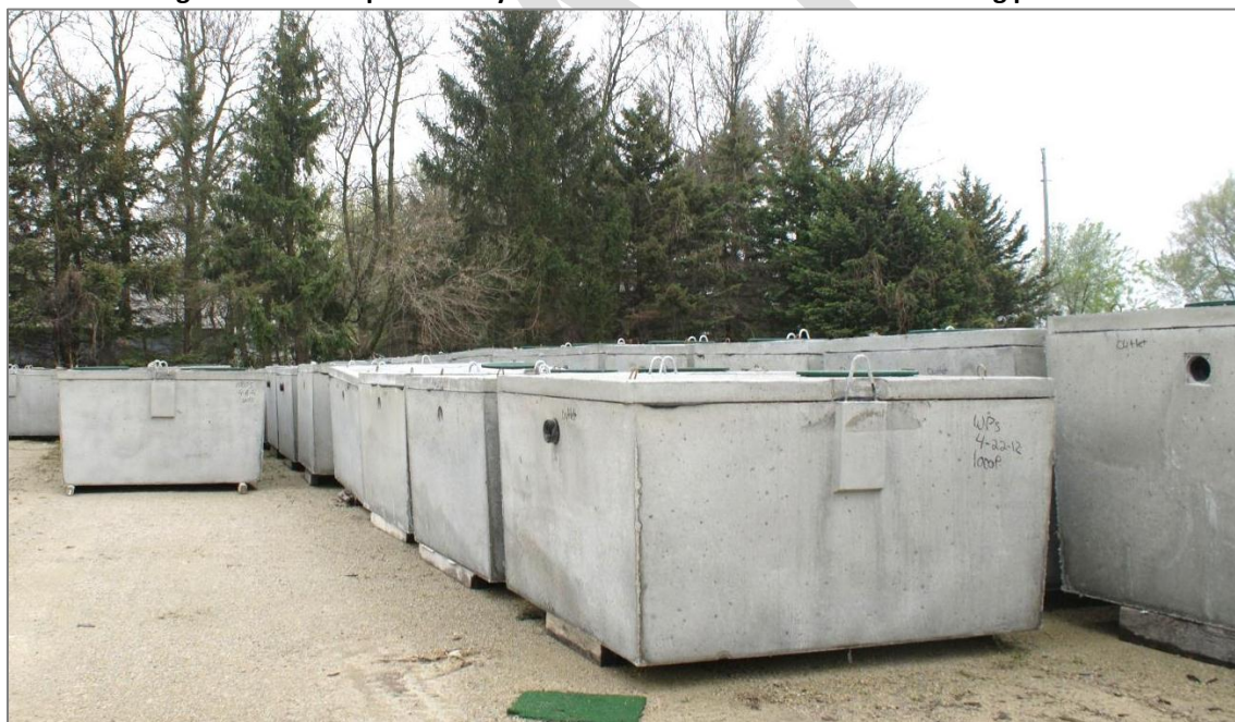
Photo 4. Sewage tanks lined up and ready for use at a concrete tank manufacturing plant in Minnesota.
