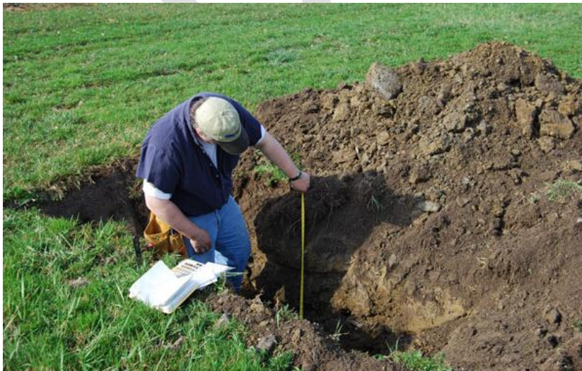
Photo 1. Describing and verifying soils in a shallow test pit using a Munsell color book to identify soil colors and determine depth to seasonal saturation.
