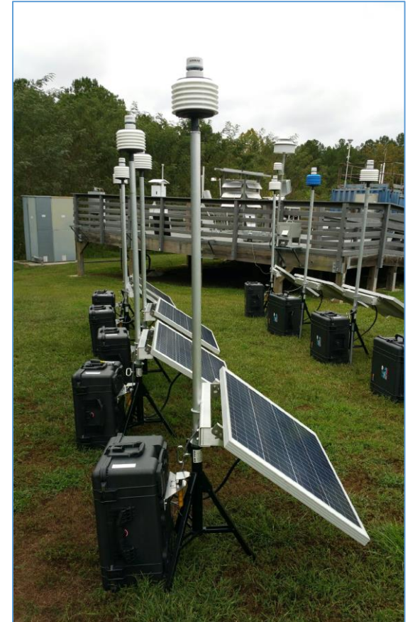
e.g., community air sensor system developed by EPA Office of Research and Development
