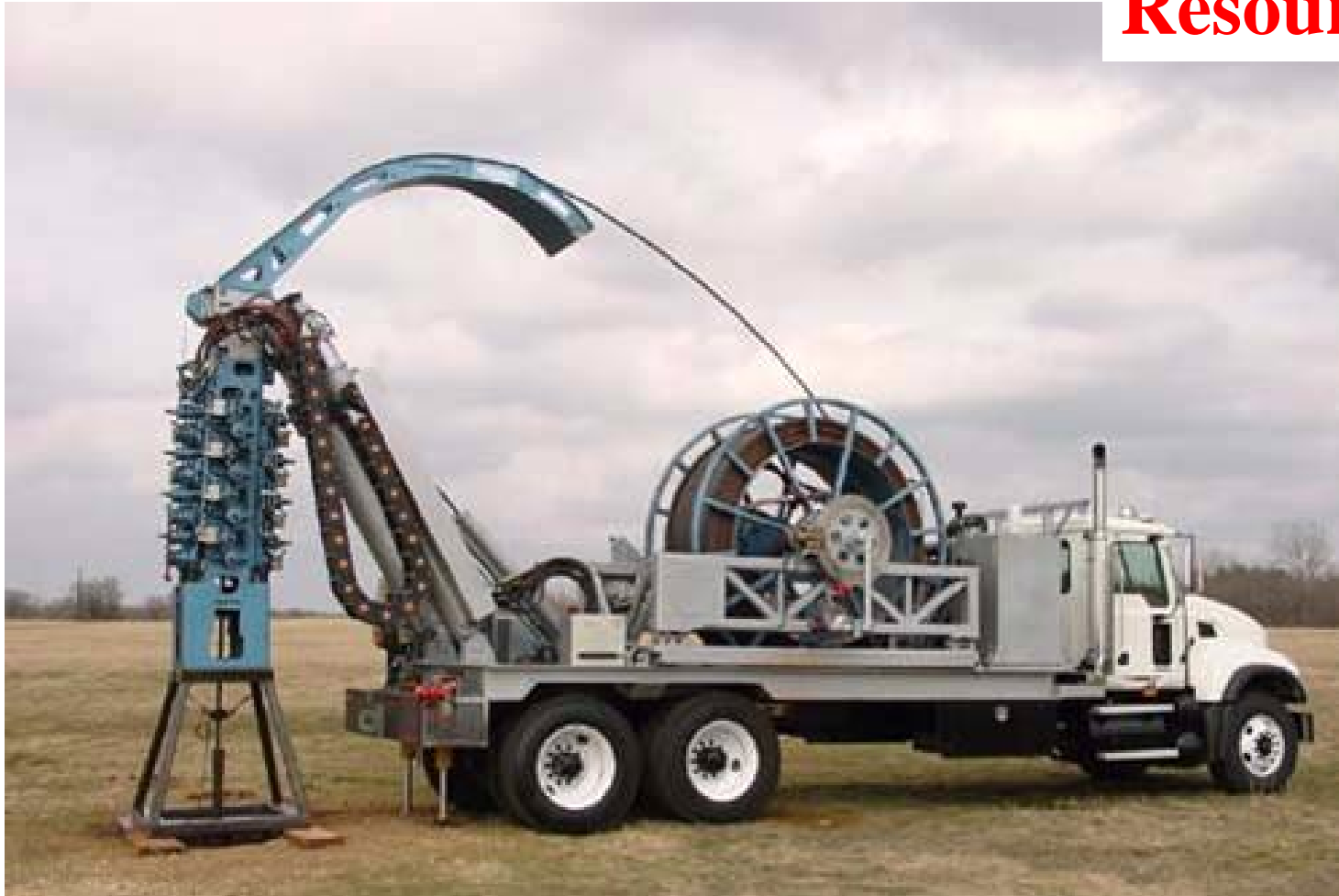
Hybrid coiled-tubing drilling rig (courtesy of DOE and Tom Gipson – New Force Energy Services, Inc)
