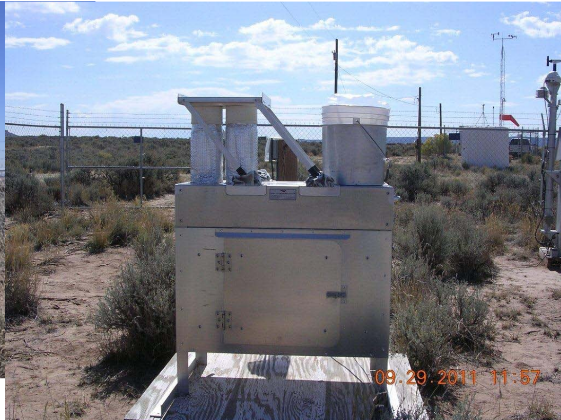
Navajo Lake Site, NM Monitor type: Wet Deposition Mercury Study duration: Ongoing
