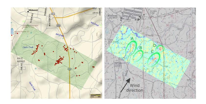
Results of grid-pattern survey of a partially abandoned oil field. Areas marked as A,B,C and D represent identified plumes.
