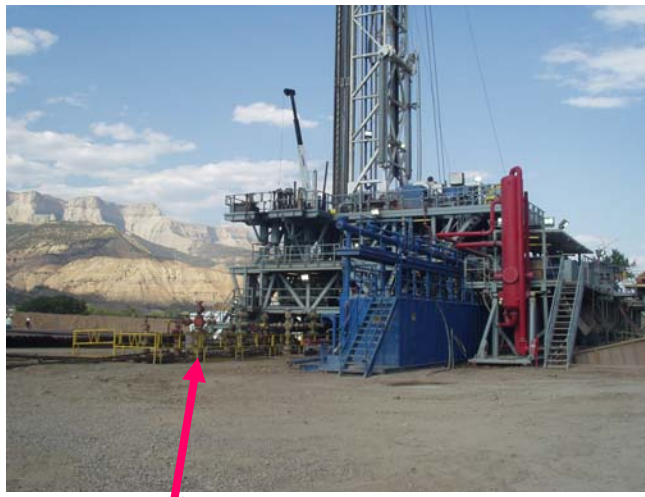
Two rows of four wells closely spaced.
