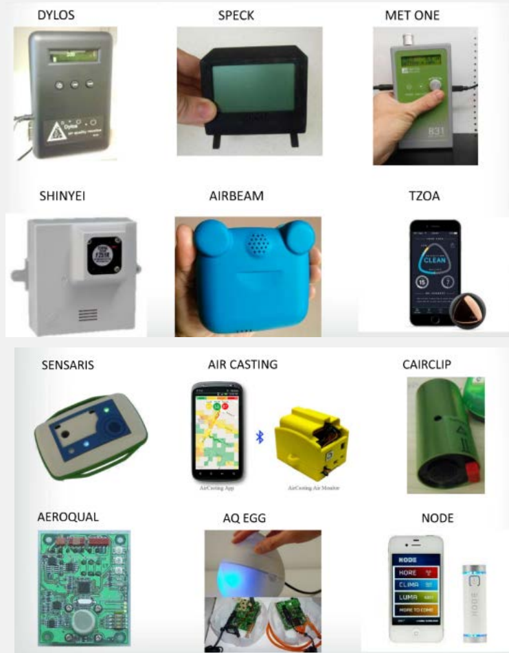
Examples of “Low-Cost” (<$2500) PM and Gas Sensors Thanks to Ron Williams, EPA
