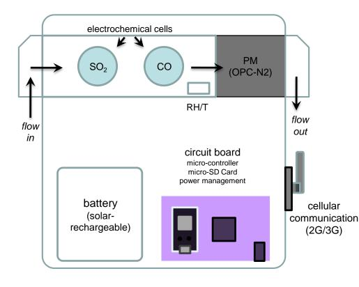
Electrochemical cells for SO<sub>2</sub> and CO (anthropogenic tracer)
