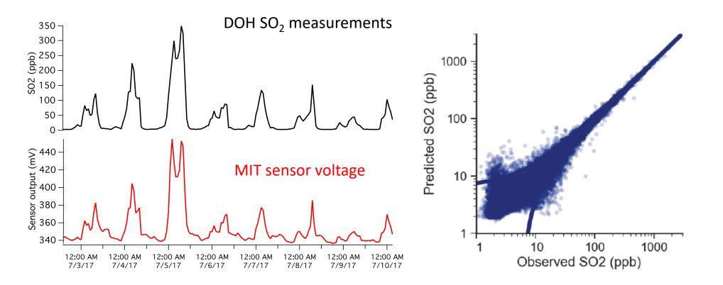
Excellent predictive power (to within 7 ppb  $SO_2$ ) No evidence of degradation over ~6 months Fall 2017-spring 2018: Design next generation node (CO, PM, improved power management)
