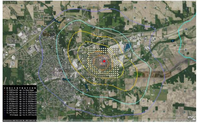
Figure 15. Predicted 99<sup>th</sup> Percentile Daily Maximum 1-Hour SO<sub>2</sub> Concentrations Averaged Over Five Years for the Area of Analysis for the Huntington County Area (Full Extent)
