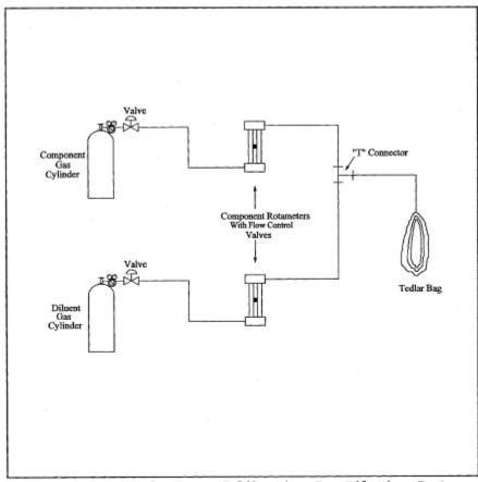
Figure 18-5. Single-Stage Calibration Gas Dilution System.
