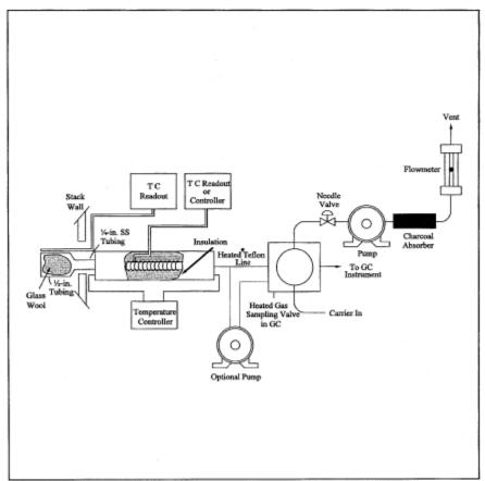
Figure 18-12. Direct Interface Sampling System.
