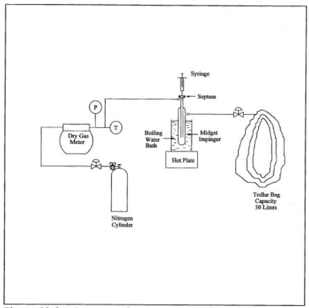
Figure 18-8. Apparatus for Preparation of Liquid Materials.
