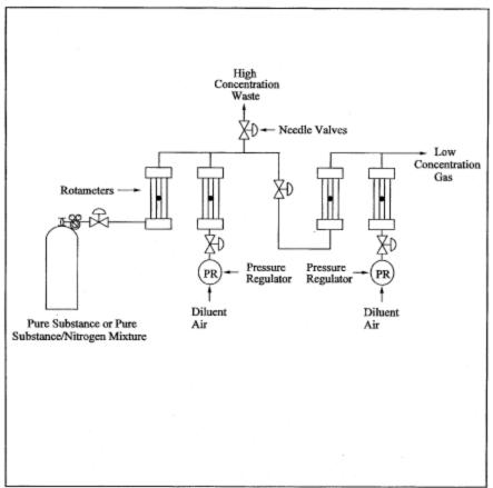
Figure 18-6. Two-Stage Dilution Apparatus.
