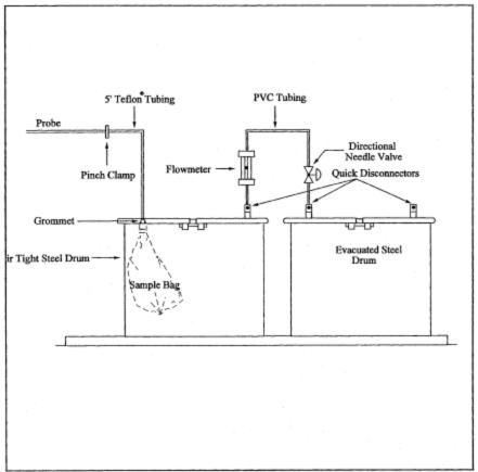
Figure 18-9a. Explosion Risk Gas Sampling Method.
