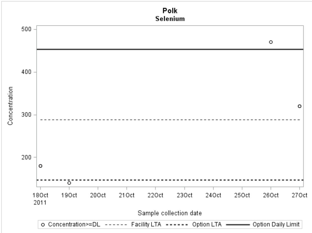
Figure A7.35 Selenium daily limitation and daily concentrations ( $\mu\text{g/L}$ ) at Wabash River used to calculate the limitations for the vapor-compression evaporation treatment technology option for gasification wastewater
