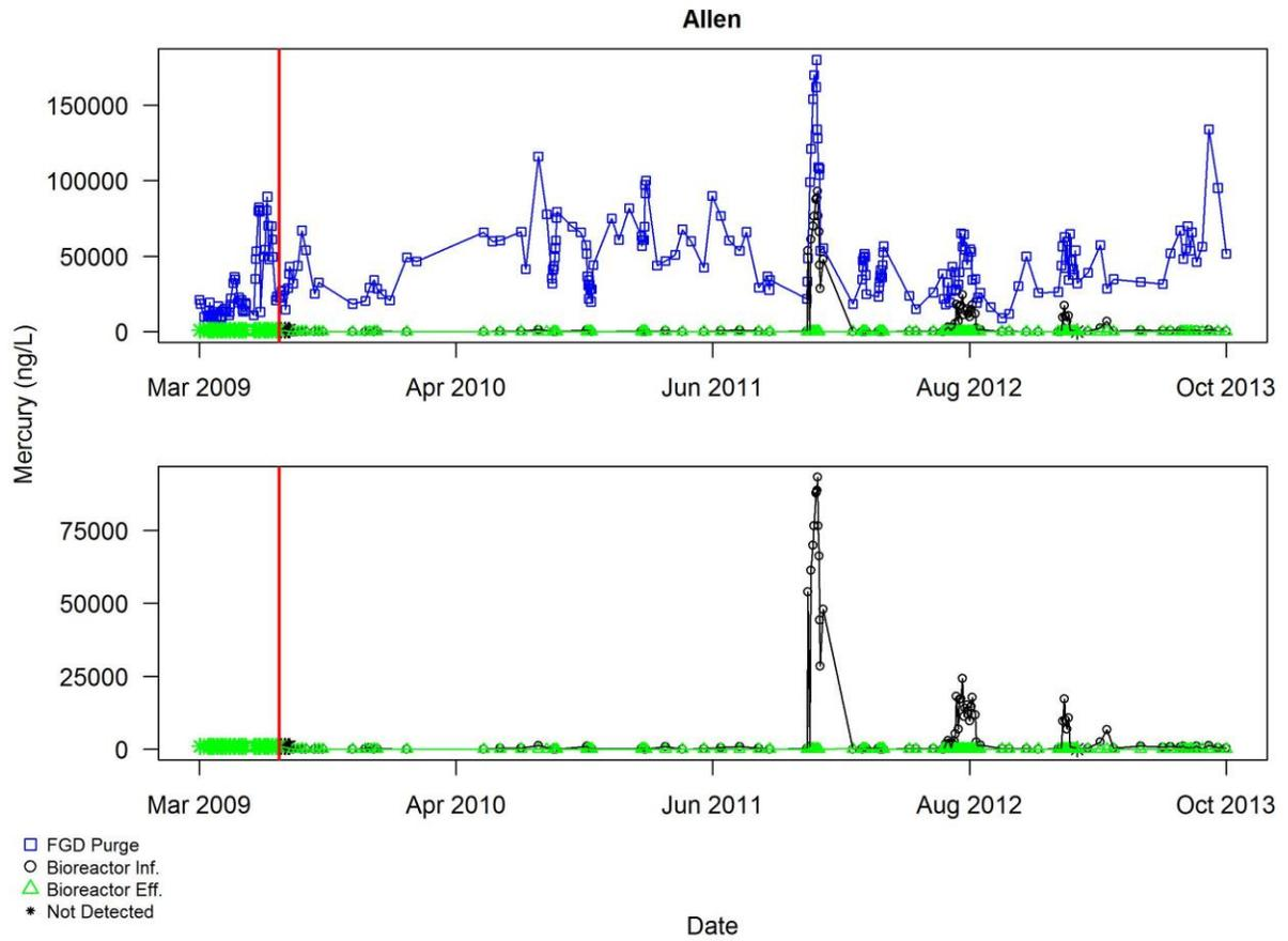
Figure A3.1.8 Plot of self-monitoring data for mercury (ng/L) for Allen after exclusions other than commissioning period described in Section 3.2 and superimposed with smooth curves using LOWESS. The red vertical line indicates the end of the commissioning period
