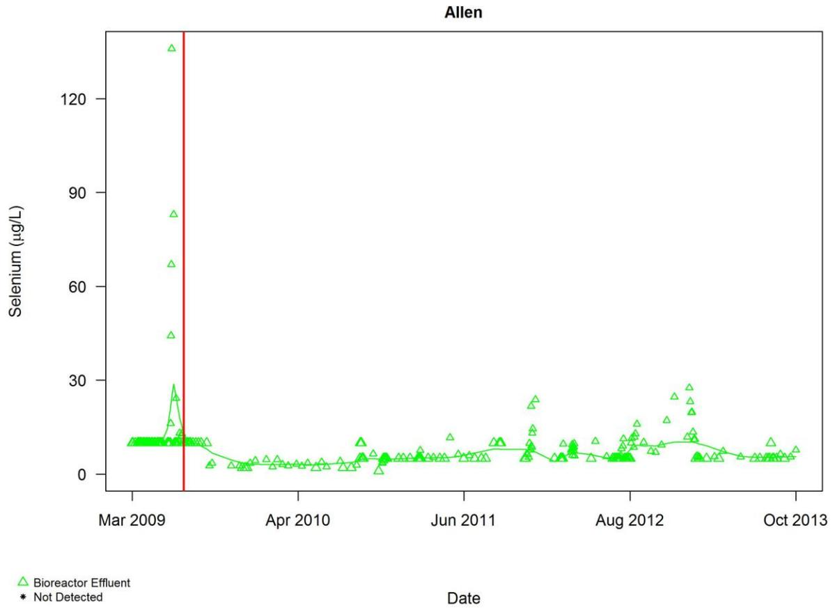
Figure A3.1.19 Plot of self-monitoring data for selenium ( $\mu\text{g/L}$ ) for Allen after exclusions other than commissioning period described in Section 3.2, bioreactor effluent only. The red vertical line indicates the end of the commissioning period
