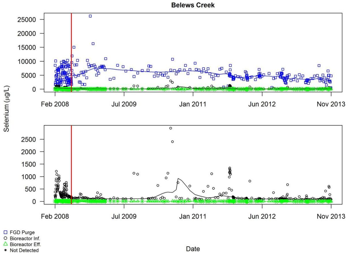
Figure A3.2.17 Plot of all self-monitoring data for selenium ( $\mu\text{g/L}$ ) for Belews Creek, bioreactor effluent only. The red vertical line indicates the end of the commissioning period
