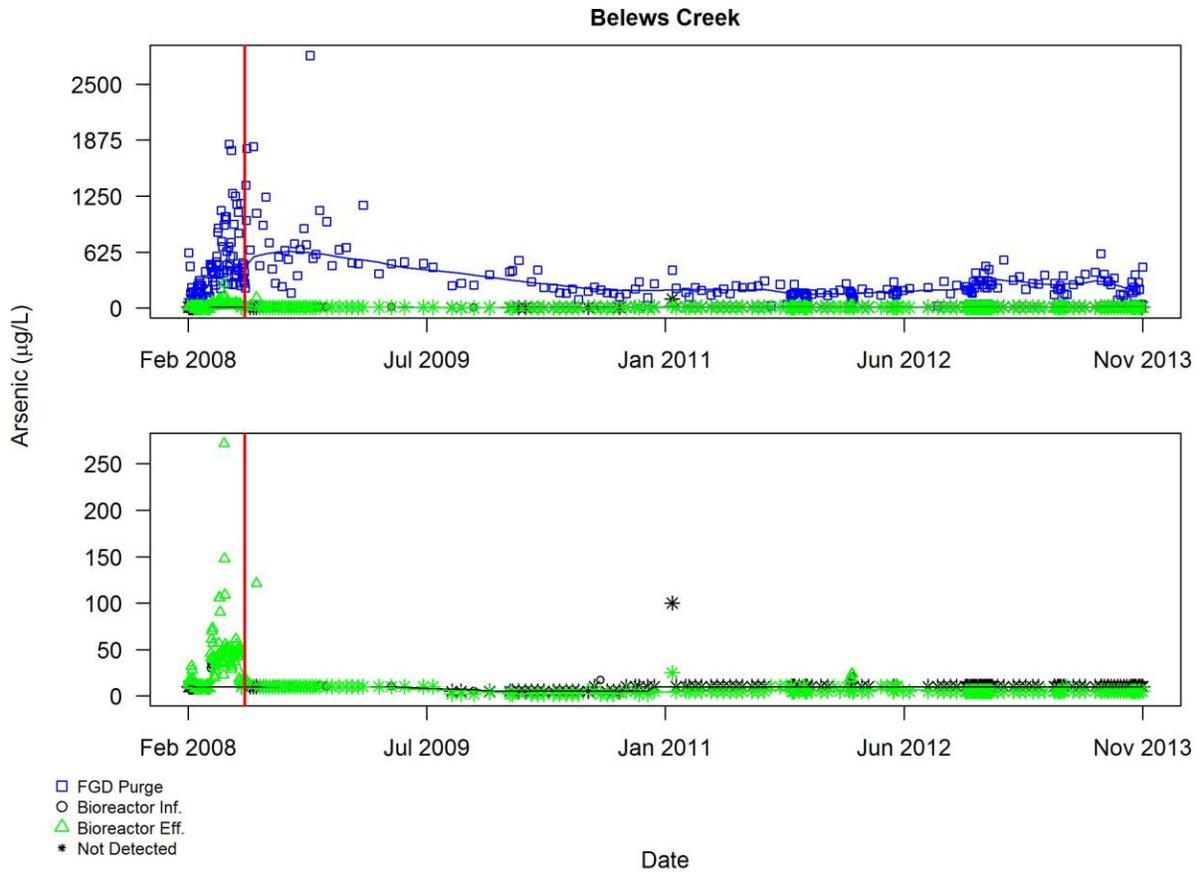
Figure A3.2.3 Plot of self-monitoring data for arsenic ( $\mu\text{g/L}$ ) for Belews Creek after exclusions other than commissioning period described in Section 3.2. The red vertical line indicates the end of the commissioning period
