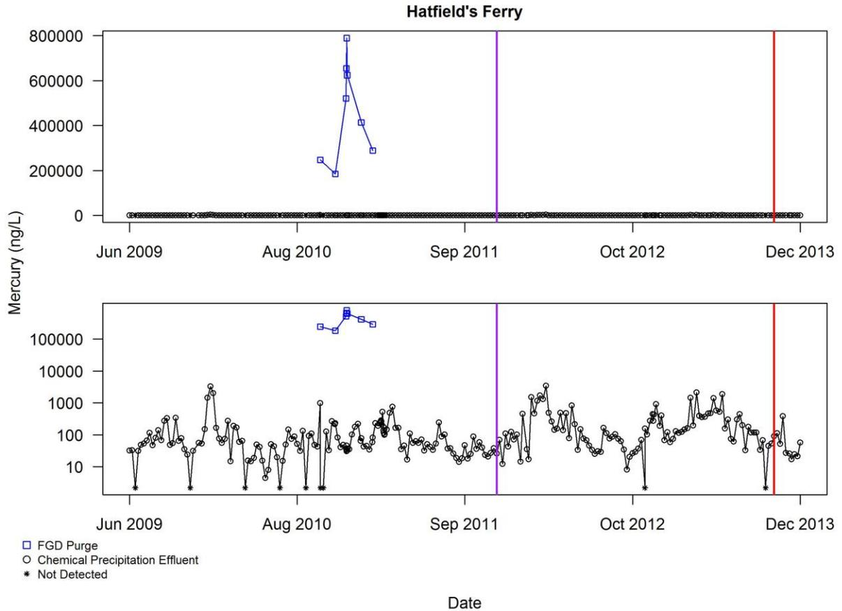
**Figure A4.1.4 Chemical precipitation effluent data of mercury for Hatfield's Ferry, prior to excluding any data for reasons described in Section 3.2. Pollutant concentrations are shown on a linear scale in the upper plot, log scale in the lower plot. The purple vertical line indicates the point when the plant changed analytical laboratories, and the red vertical line indicates the start of decommissioning period**
