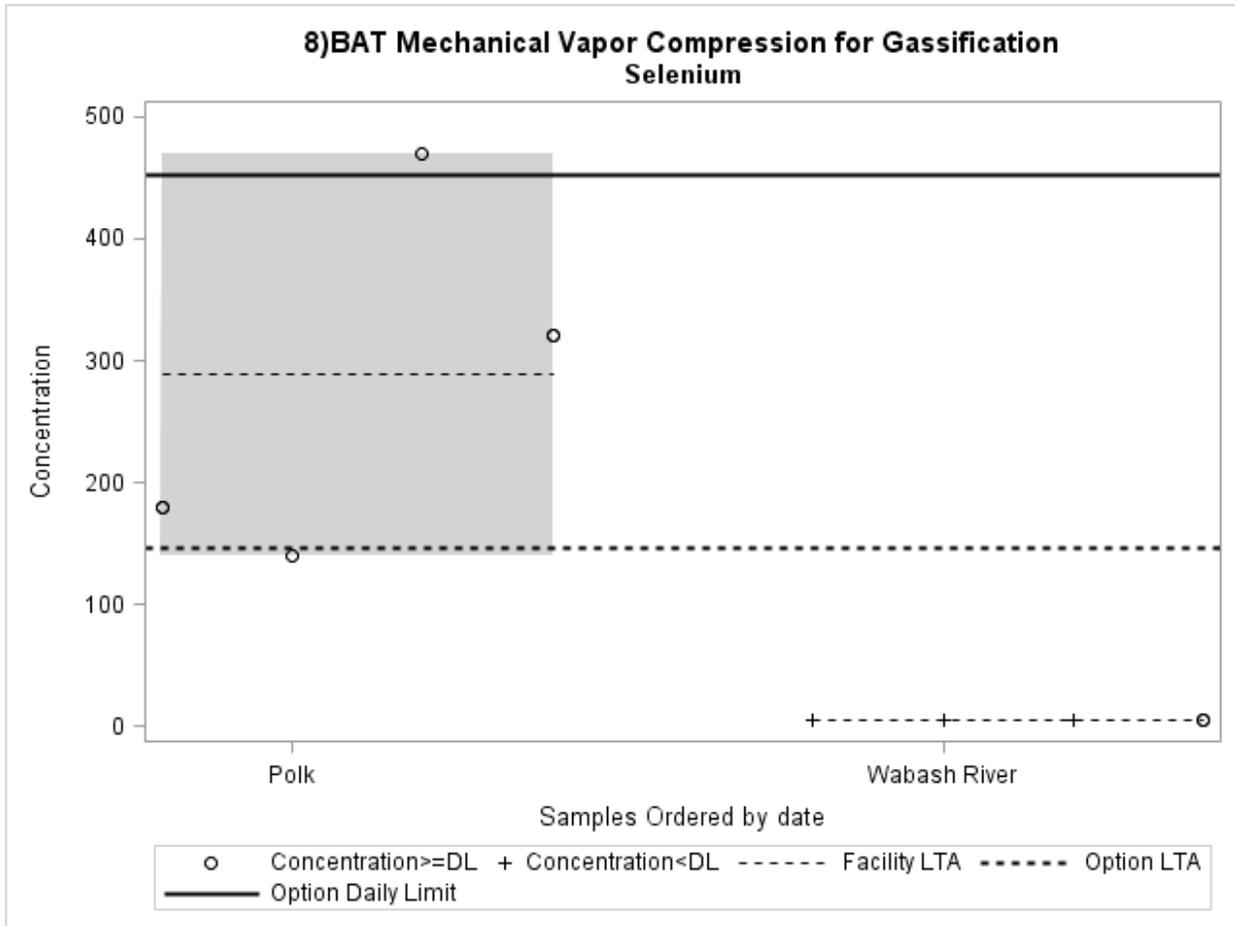
Figure A7.34 Selenium daily limitation and daily concentrations ( $\mu\text{g/L}$ ) at Polk used to calculate the limitations for the vapor-compression evaporation treatment technology option for gasification wastewater
