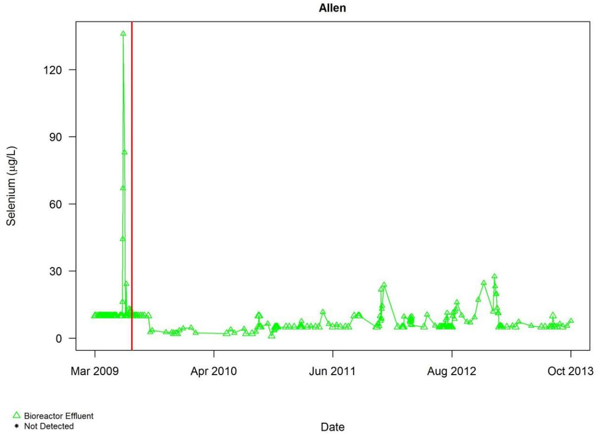
Figure A3.1.20 Plot of self-monitoring data for selenium ( $\mu\text{g/L}$ ) for Allen after exclusions other than commissioning period described in Section 3.2 and superimposed with smooth curves using LOWESS,, bioreactor effluent only. The red vertical line indicates the end of the commissioning period
