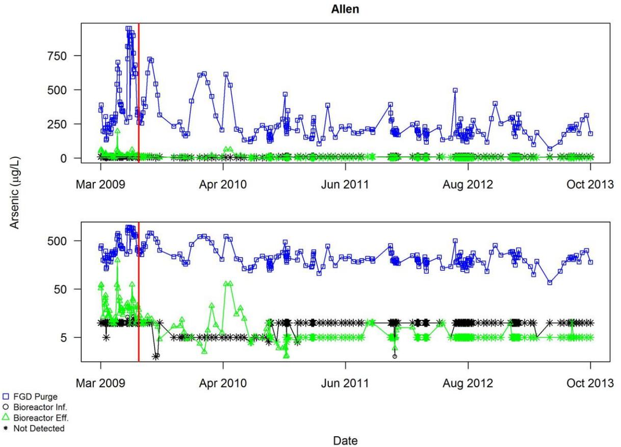
**Figure A4.5.2 Bioreactor influent and Bioreactor effluent data of arsenic for Allen, prior to excluding any data for reasons described in Section 3.2. Pollutant concentrations are shown on a linear scale in the upper plot, log scale in the lower plot. The red vertical line indicates the end of the commissioning period**
