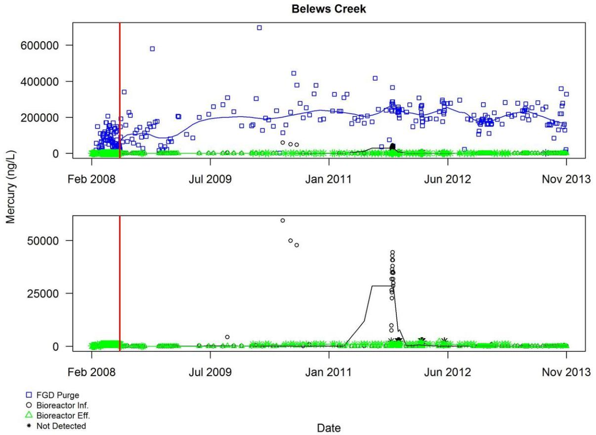
Figure A3.2.7 Plot of self-monitoring data for mercury (ng/L) for Belews Creek after exclusions other than commissioning period described in Section 3.2. The red vertical line indicates the end of the commissioning period
