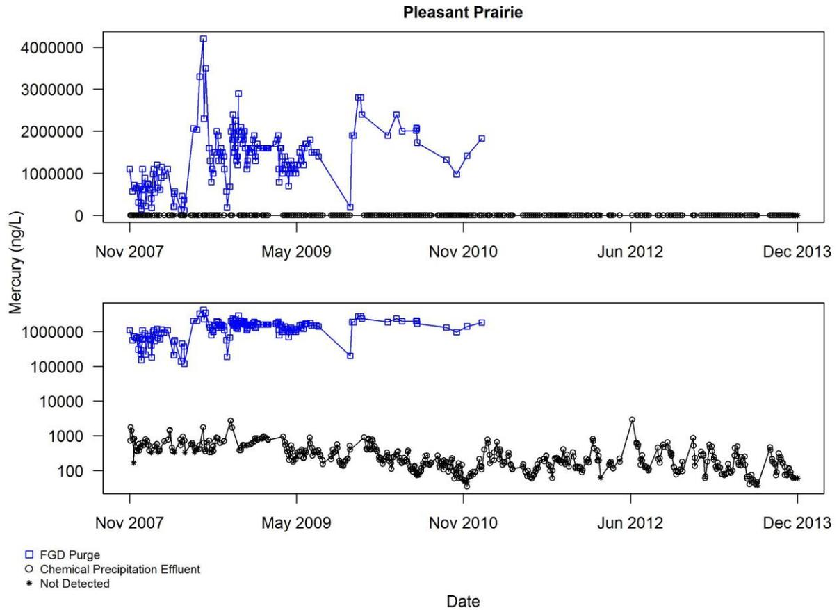
**Figure A4.4.4 Chemical precipitation effluent data of mercury for Pleasant Prairie, prior to excluding any data for reasons described in Section 3.2. Pollutant concentrations are shown on a linear scale in the upper plot, log scale in the lower plot**
