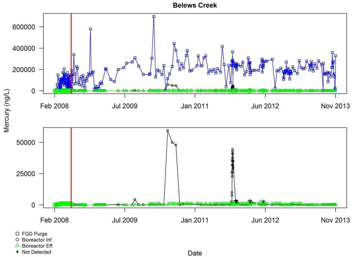
Figure A3.2.6 Plot of all self-monitoring data for mercury (ng/L) for Belews Creek superimposed with smooth curves using LOWESS. The red vertical line indicates the end of the commissioning period
