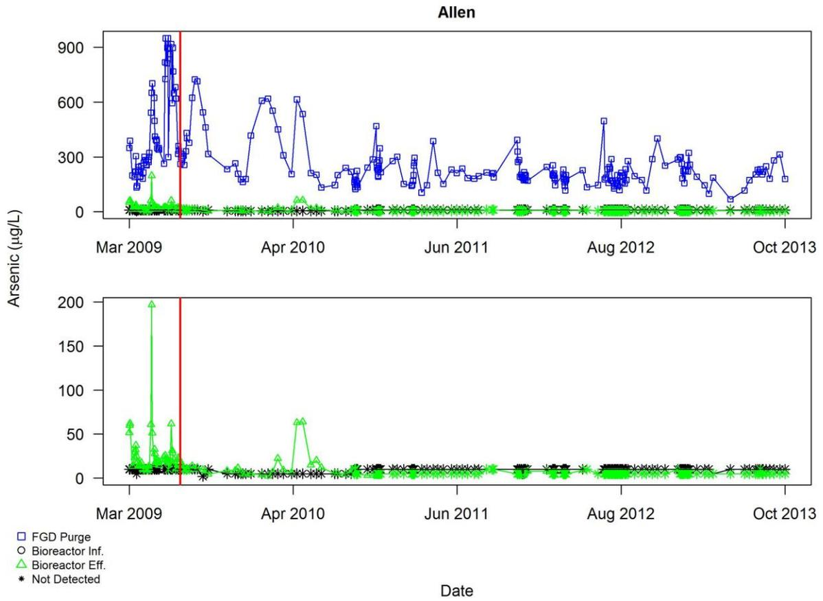
Figure A3.1.2 Plot of all self-monitoring data for arsenic ( $\mu\text{g/L}$ ) for Allen superimposed with smooth curves using LOWESS. The red vertical line indicates the end of the commissioning period
