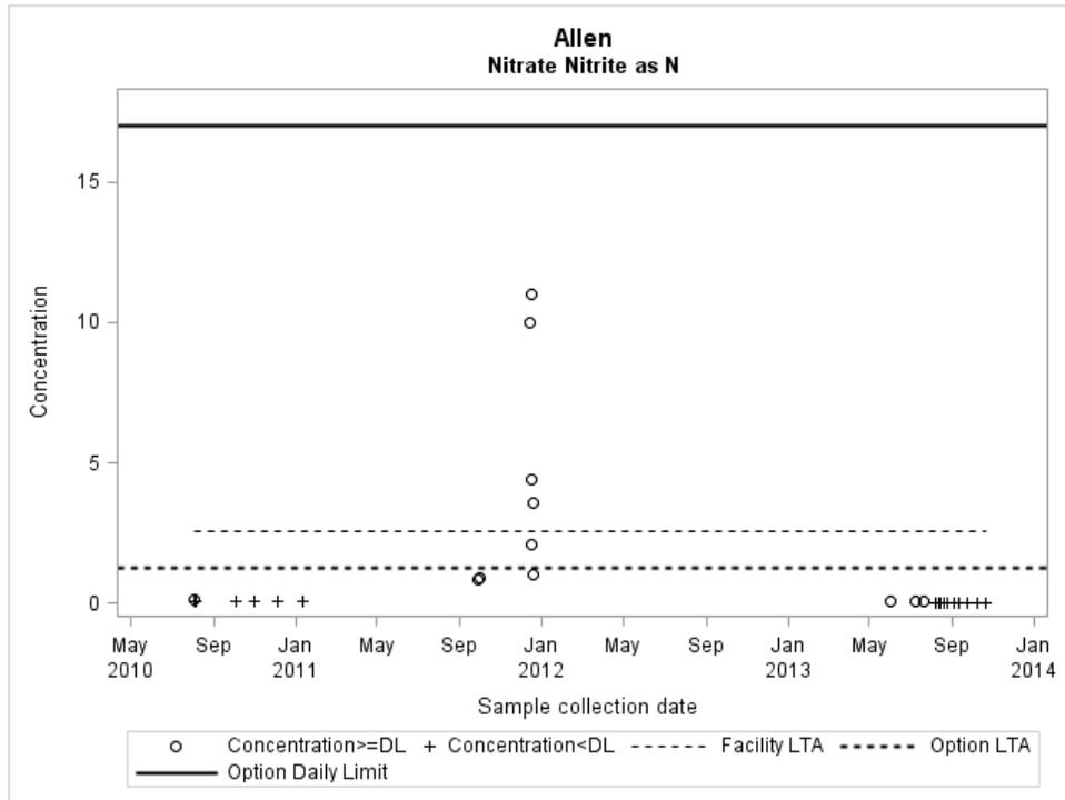
**Figure A7.19 Nitrite Nitrate as N daily limitation and daily concentrations (mg/L) at Belews Creek used to calculate the limitations for the biological treatment of FGD wastewater**
