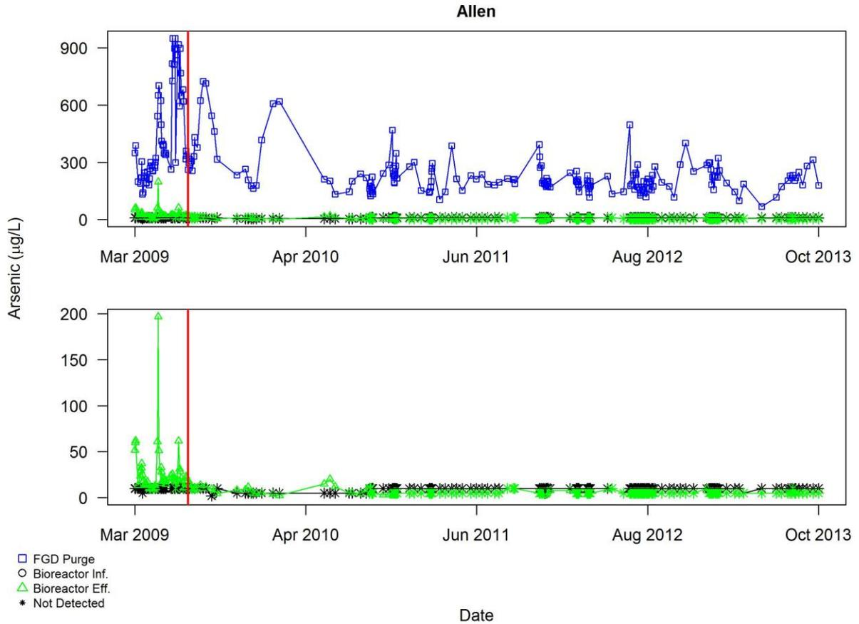
Figure A3.1.4 Plot of self-monitoring data for arsenic ( $\mu\text{g/L}$ ) for Allen after exclusions other than commissioning period described in Section 3.2 and superimposed with smooth curves using LOWESS. The red vertical line indicates the end of the commissioning period
