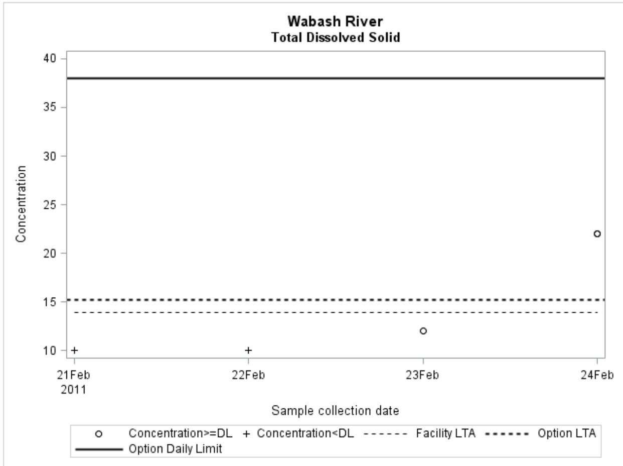
**Table A7.5** Listing of all daily values that are above the daily limits for vapor-compression evaporation treatment for gasification wastewater
