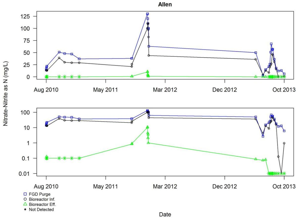
**Figure A4.5.8 Bioreactor influent and Bioreactor effluent data of Nitrate-Nitrite as N for Allen, prior to excluding any data for reasons described in Section 3.2. Pollutant concentrations are shown on a linear scale in the upper plot, log scale in the lower plot**
