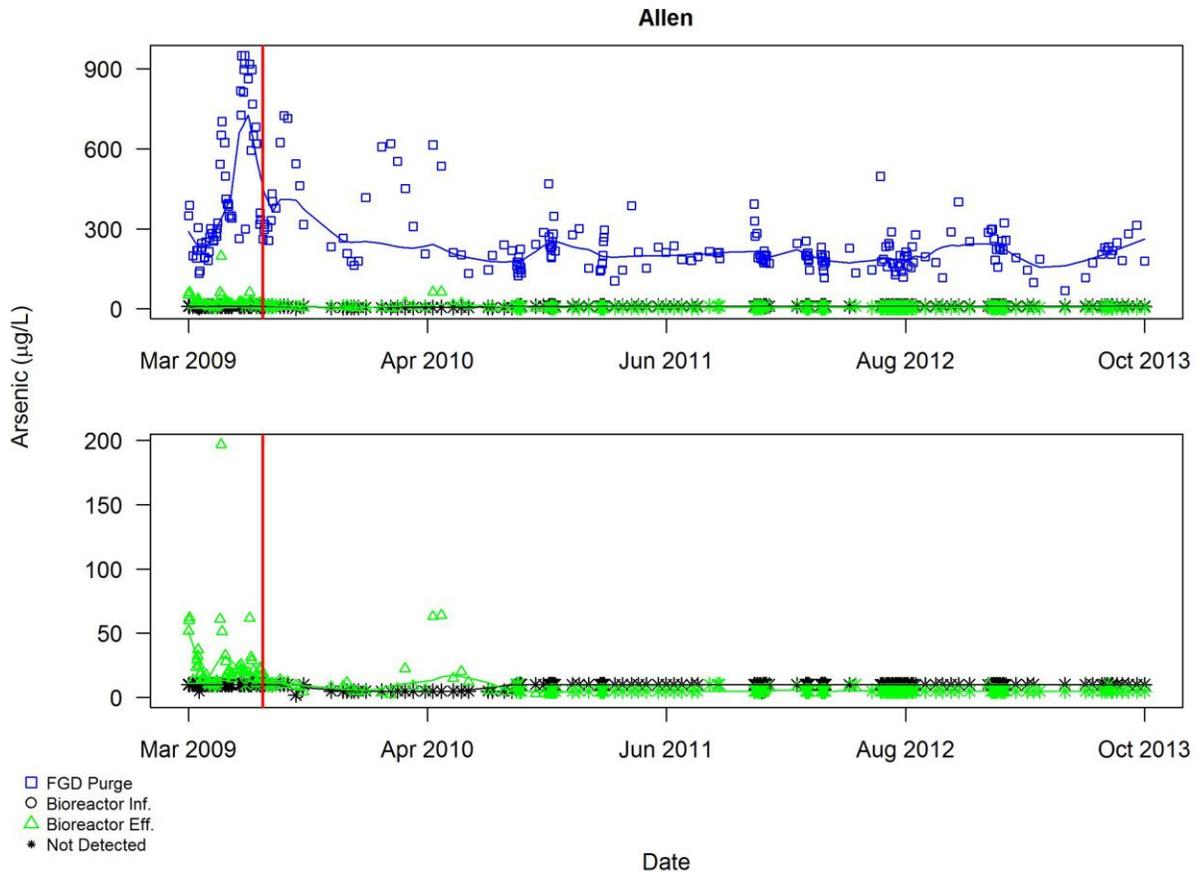
Figure A3.1.3 Plot of self-monitoring data for arsenic ( $\mu\text{g/L}$ ) for Allen after exclusions other than commissioning period described in Section 3.2. The red vertical line indicates the end of the commissioning period
