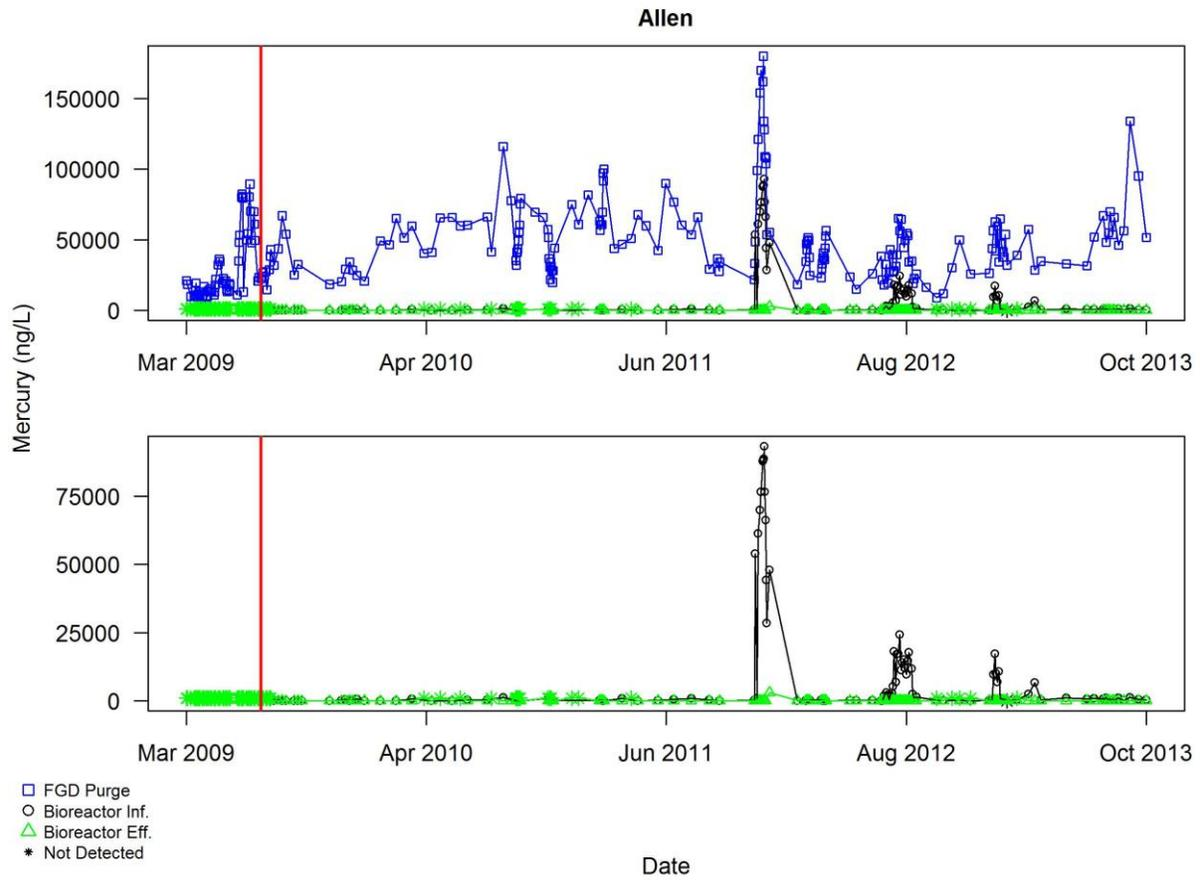
Figure A3.1.6 Plot of all self-monitoring data for mercury (ng/L) for Allen superimposed with smooth curves using LOWESS. The red vertical line indicates the end of the commissioning period
