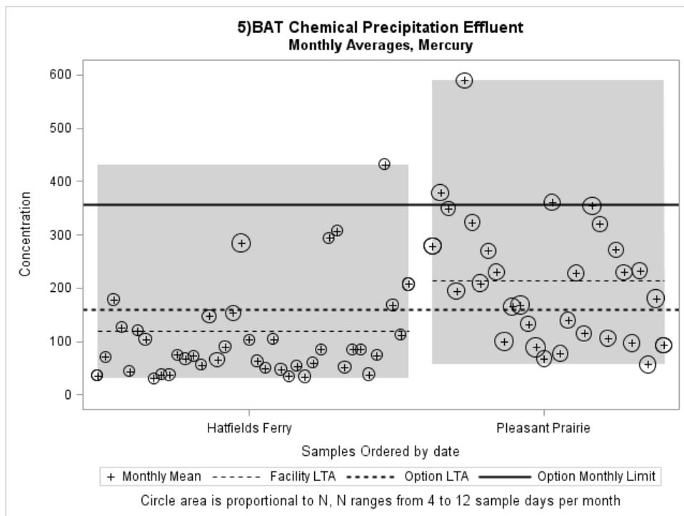
**Figure A7.15 Mercury monthly limitation and monthly average concentrations (ng/L) at Hatfield's Ferry for chemical precipitation treatment of FGD wastewater**
