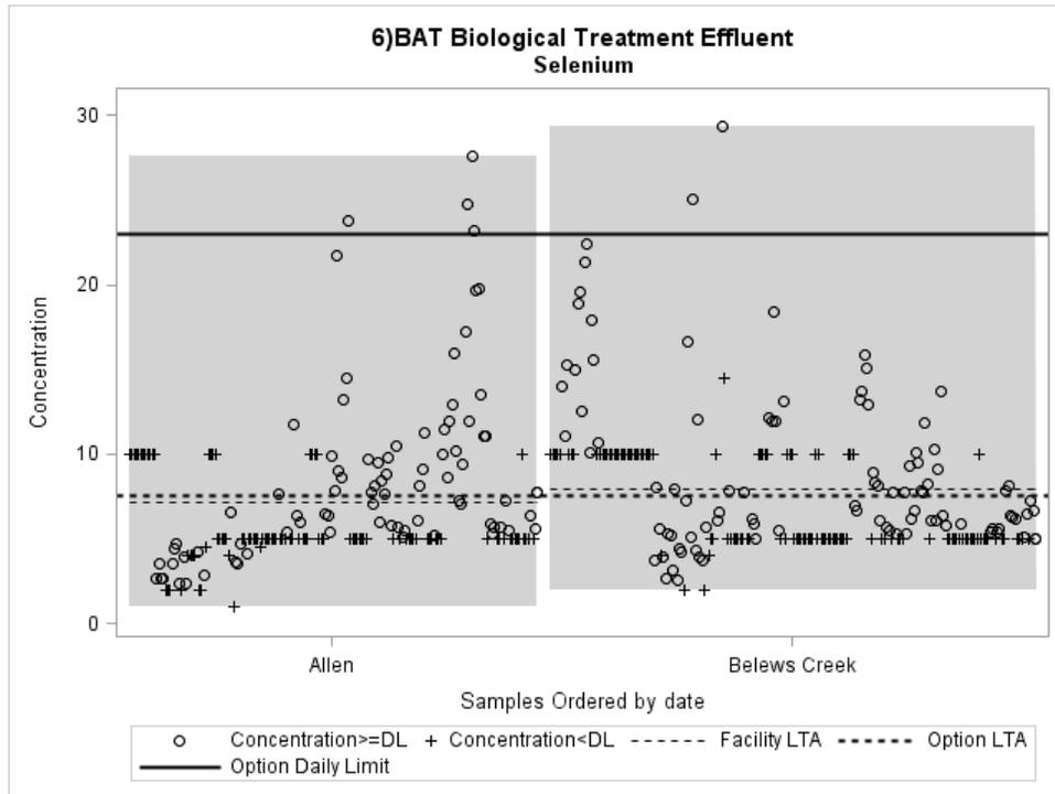
Figure A7.21 Selenium daily limitation and daily concentrations ( $\mu\text{g/L}$ ) at Allen used to calculate the limitations for biological treatment of FGD wastewater
