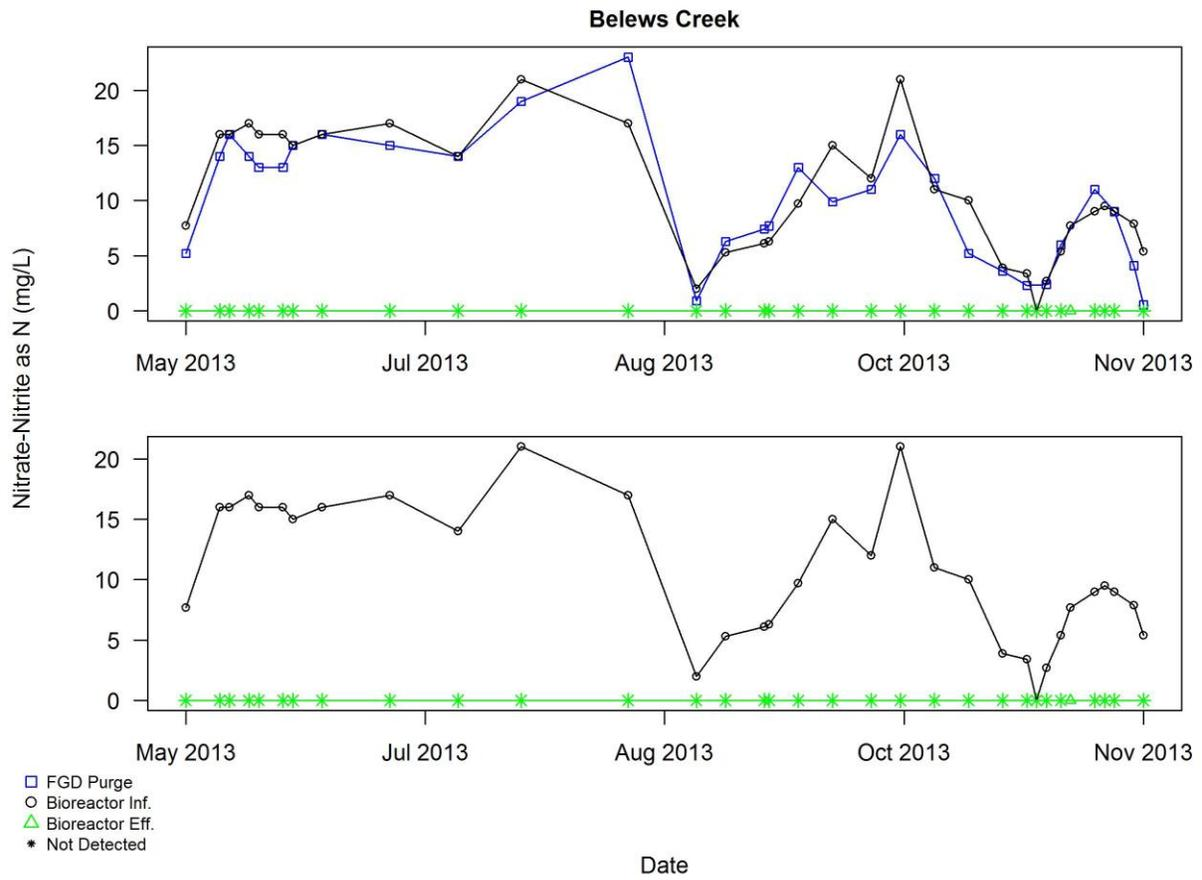
Figure A3.2.10 Plot of all self-monitoring data for Nitrate-Nitrite as N (mg/L) for Belews Creek superimposed with smooth curves using LOWESS
