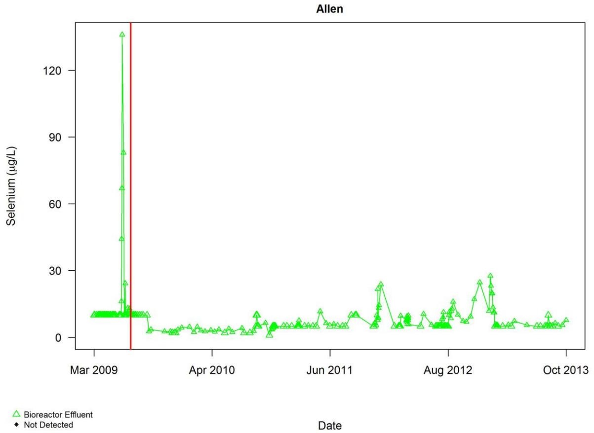
Figure A3.1.18 Plot of all self-monitoring data for selenium ( $\mu\text{g/L}$ ) for Allen superimposed with smooth curves using LOWESS, bioreactor effluent only. The red vertical line indicates the end of the commissioning period
