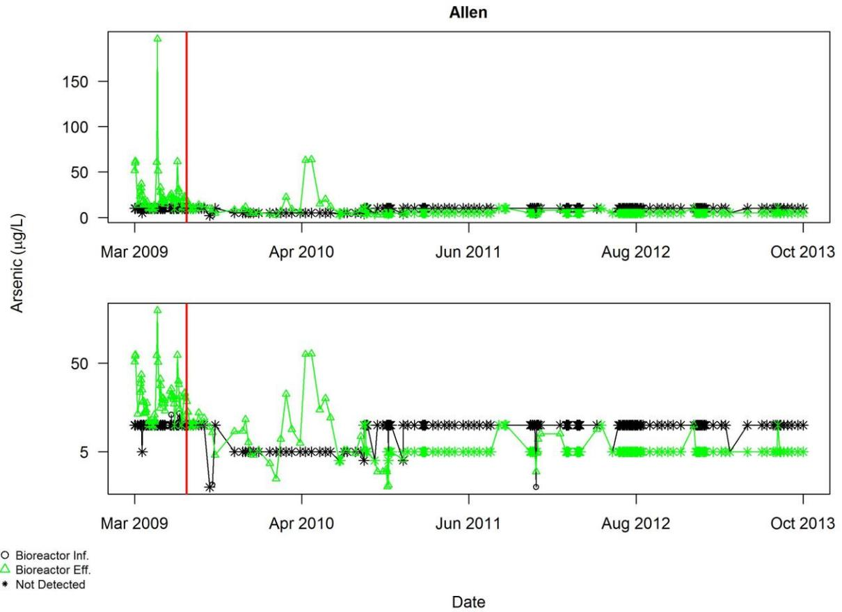
Figure A4.5.3 Bioreactor effluent data of arsenic for Allen, prior to excluding any data for reasons described in Section 3.2. Pollutant concentrations are shown on a linear scale in the upper plot, log scale in the lower plot. The red vertical line indicates the end of the commissioning period
