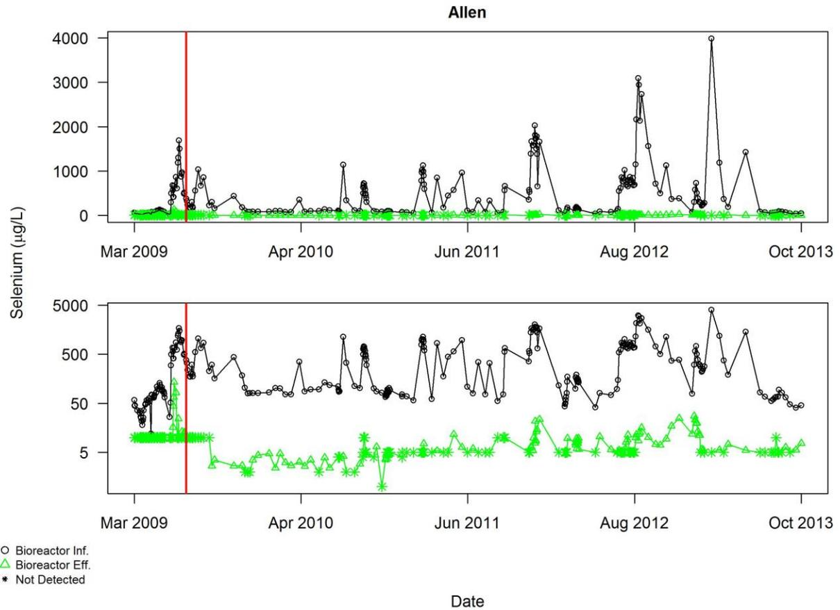
Figure A4.5.12 Bioreactor effluent data of selenium for Allen, prior to excluding any data for reasons described in Section 3.2. Pollutant concentrations are shown on a linear scale in the upper plot, log scale in the lower plot. The red vertical line indicates the end of the commissioning period
