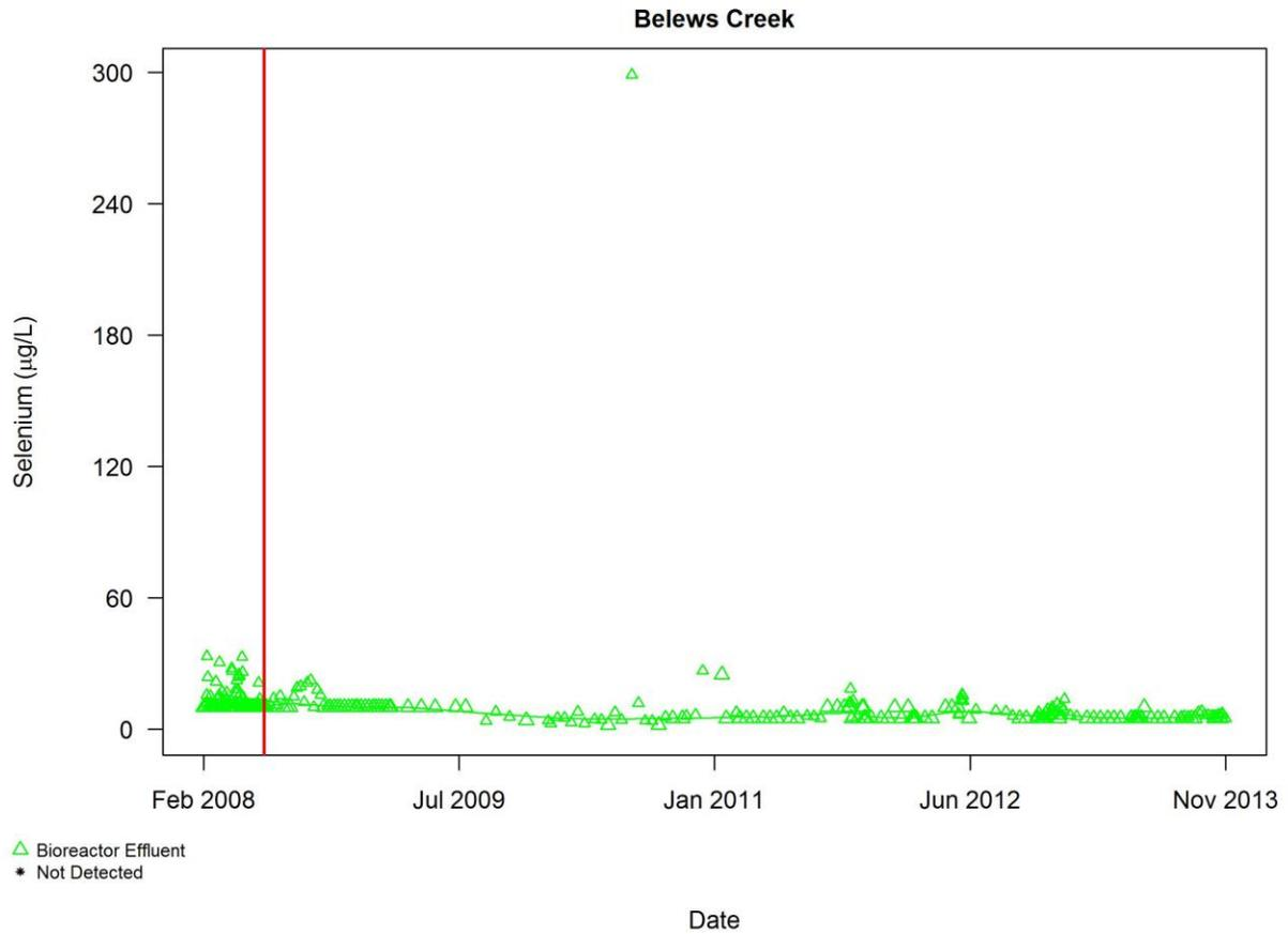
Figure A3.2.20 Plot of self-monitoring data for selenium ( $\mu\text{g/L}$ ) for Belews Creek after exclusions other than commissioning period described in Section 3.2 and superimposed with smooth curves using LOWESS, bioreactor effluent only. The red vertical line indicates the end of the commissioning period
