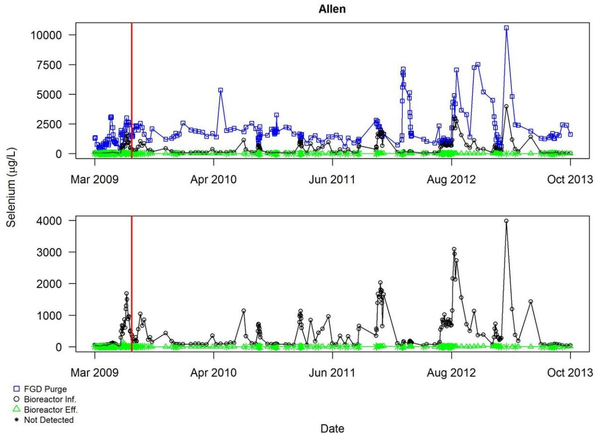
Figure A3.1.14 Plot of all self-monitoring data for selenium ( $\mu\text{g/L}$ ) for Allen superimposed with smooth curves using LOWESS. The red vertical line indicates the end of the commissioning period
