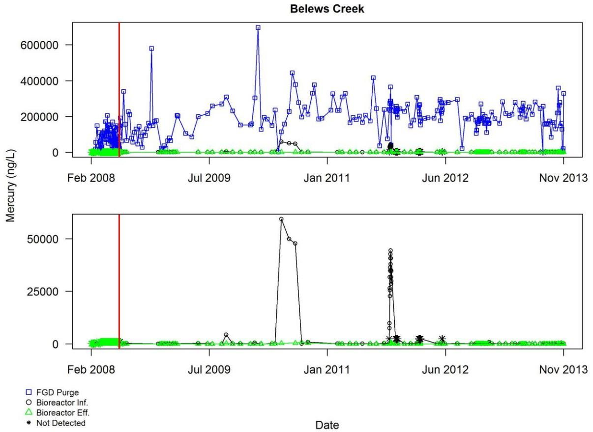
Figure A3.2.8 Plot of self-monitoring data for mercury (ng/L) for Belews Creek after exclusions other than commissioning period described in Section 3.2 and superimposed with smooth curves using LOWESS. The red vertical line indicates the end of the commissioning period
