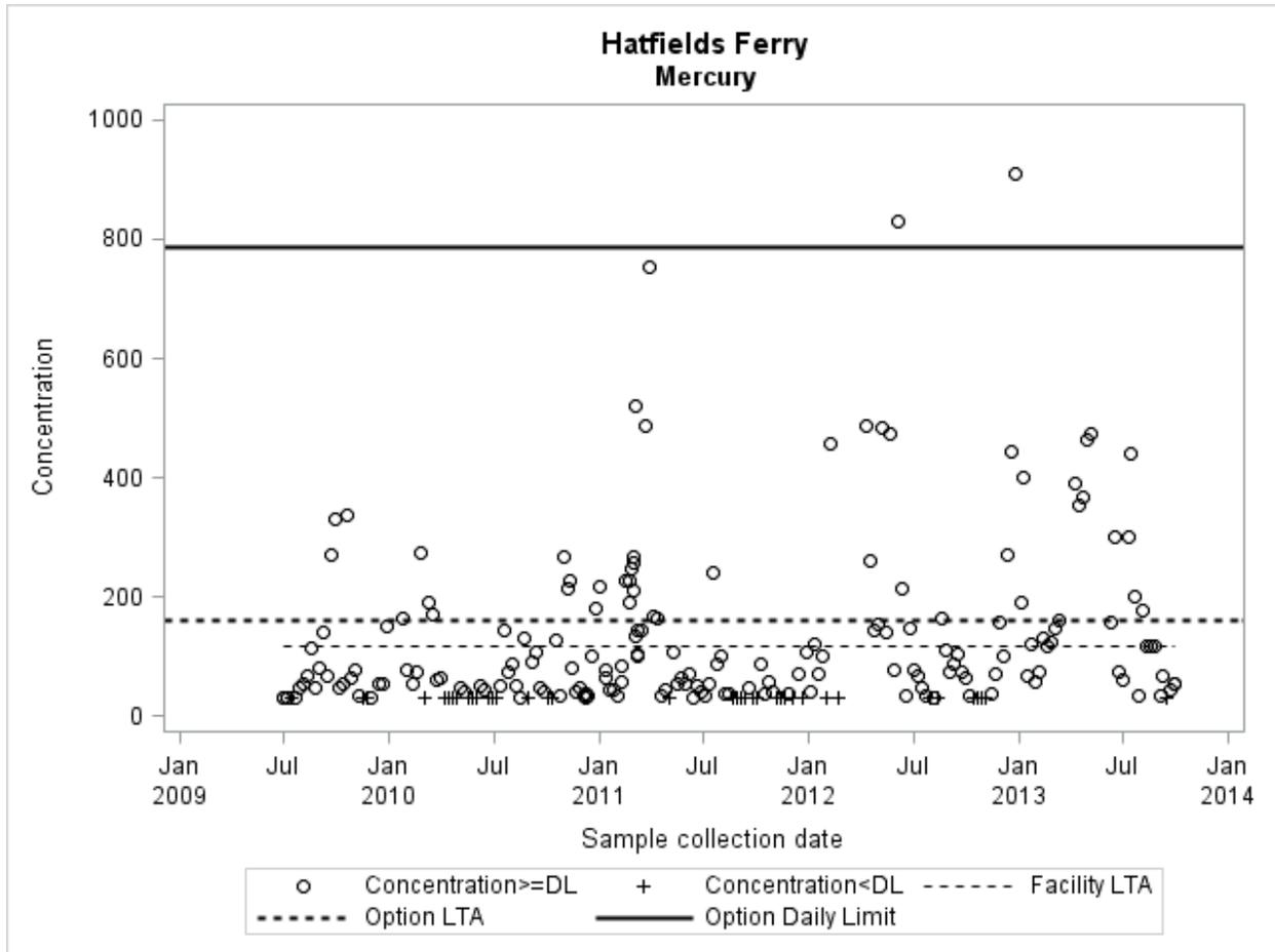
**Figure A7.8** Mercury daily limitation and daily concentrations (ng/L) at Keystone used to calculate the limitations based on chemical precipitation treatment of FGD wastewater
