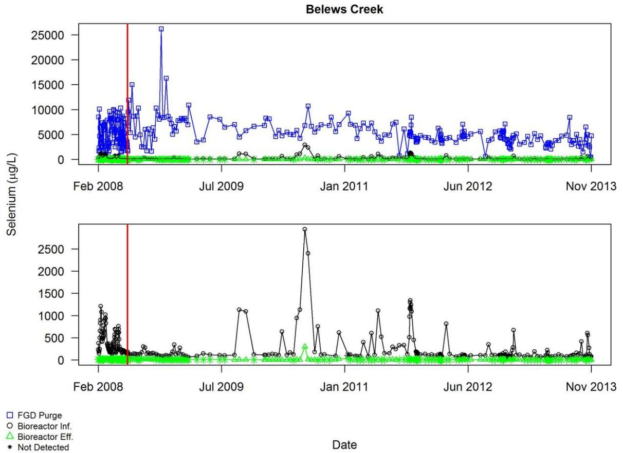
Figure A3.2.14 Plot of all self-monitoring data for selenium ( $\mu\text{g/L}$ ) for Belews Creek superimposed with smooth curves using LOWESS. The red vertical line indicates the end of the commissioning period.
