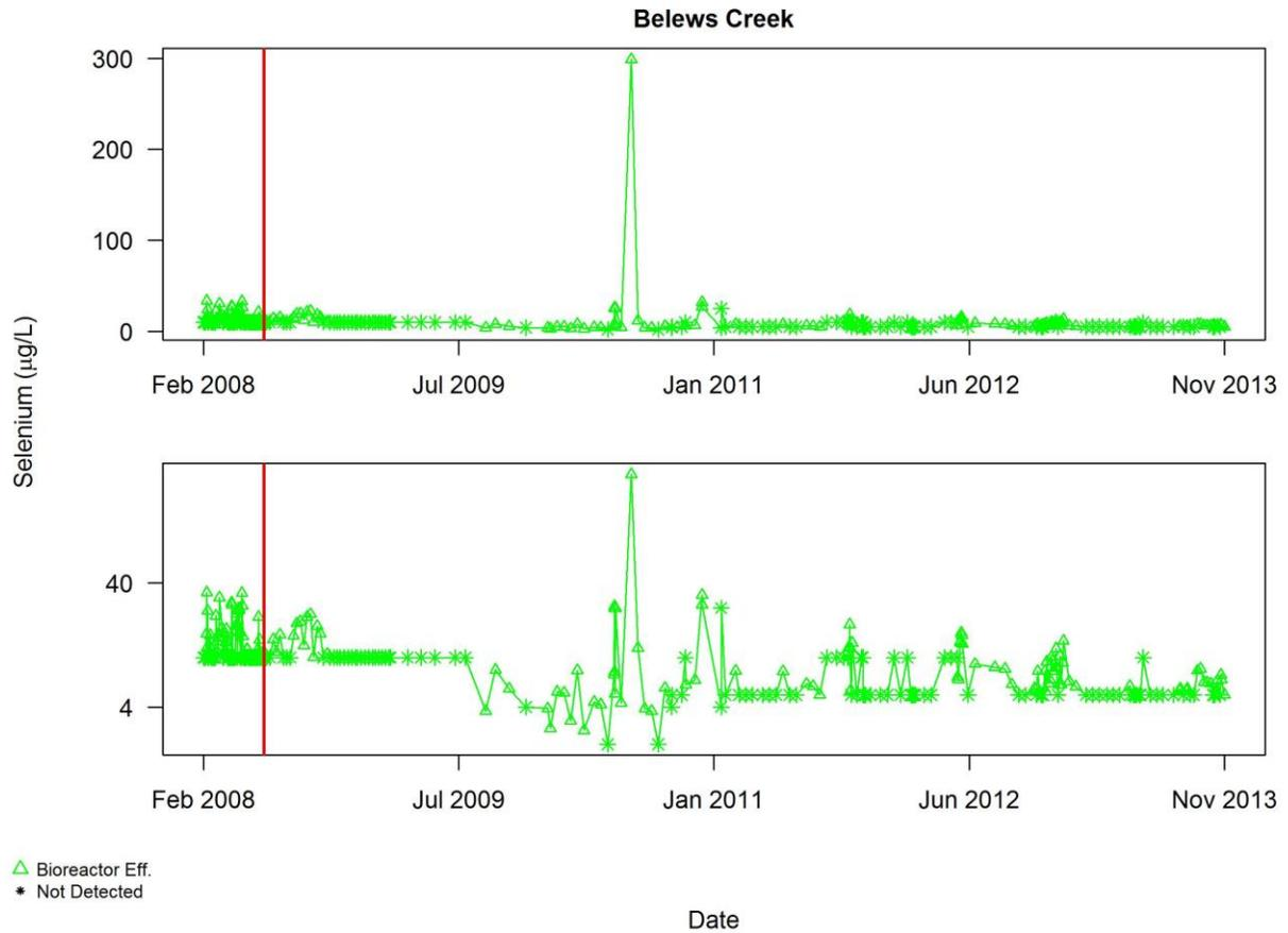
**Appendix 5. Plots to Identify Potential Outlier Observations Not Consistent with BAT/NSPS Operation of the Treatment System**
