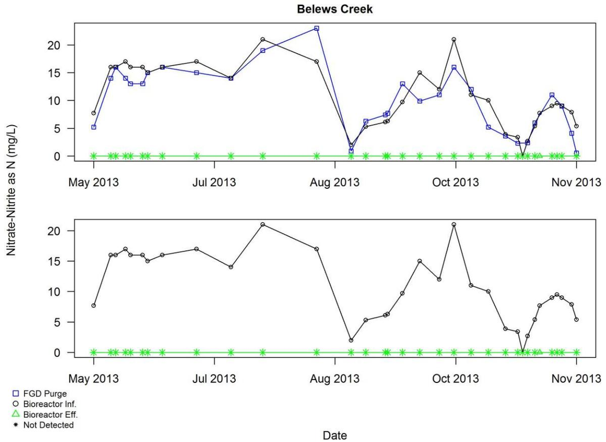
Figure A3.2.12 Plot of self-monitoring data for Nitrate-Nitrite as N (mg/L) for Belews Creek after exclusions other than commissioning period described in Section 3.2 and superimposed with smooth curves using LOWESS
