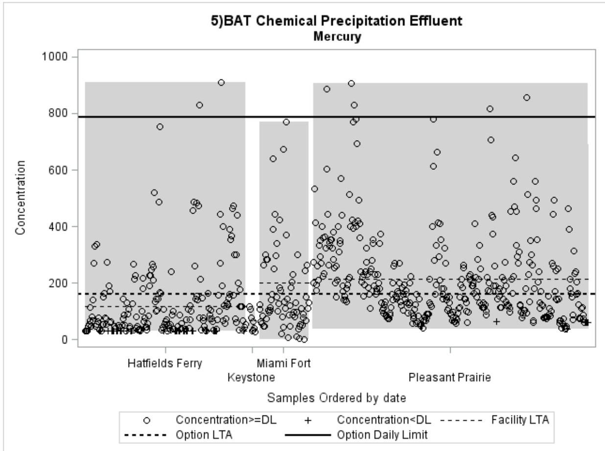
**Figure A7.7 Mercury daily limitation and daily concentrations (ng/L) at Hatfield's Ferry used to calculate the limitations based on chemical precipitation treatment of FGD wastewater**
