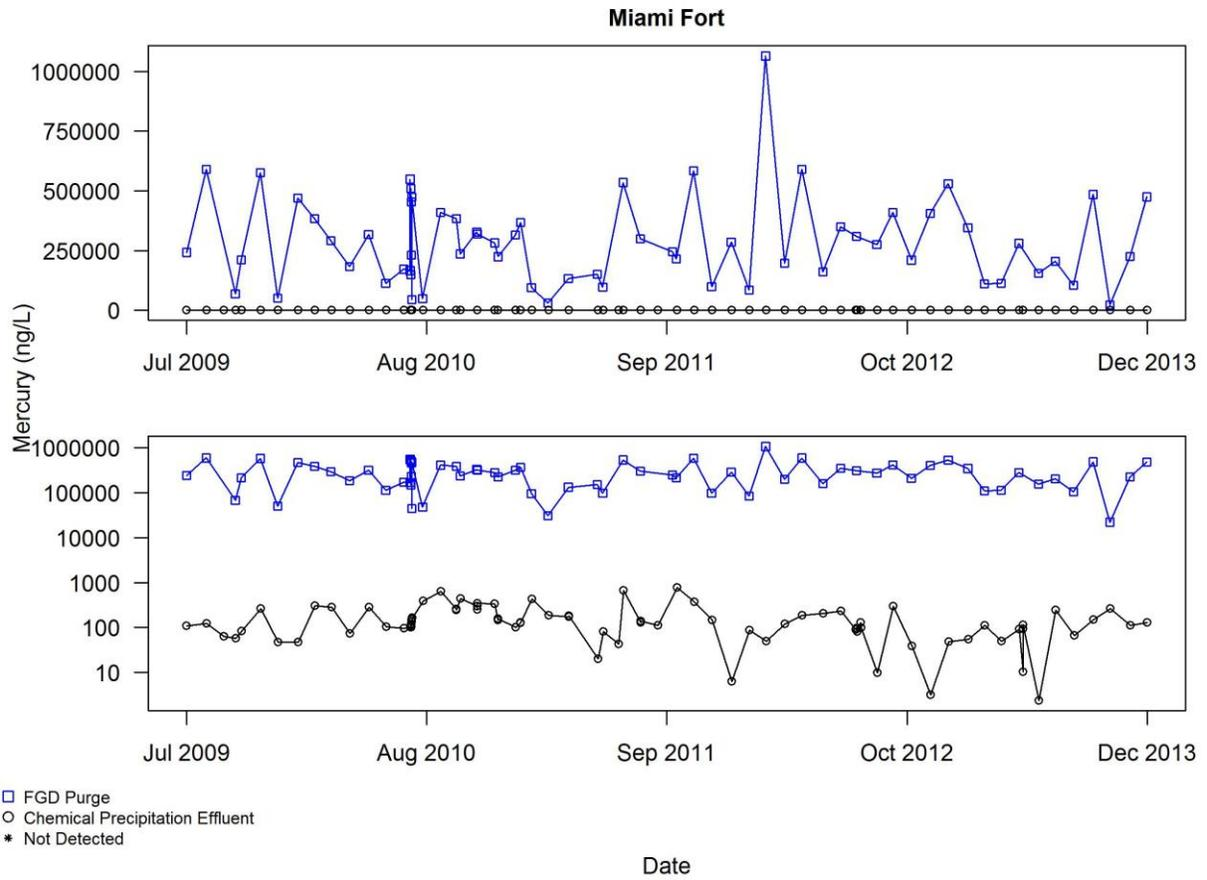
**Figure A4.3.4 Chemical precipitation effluent data of mercury for Miami Fort, prior to excluding any data for reasons described in Section 3.2. Pollutant concentrations are shown on a linear scale in the upper plot, log scale in the lower plot**
