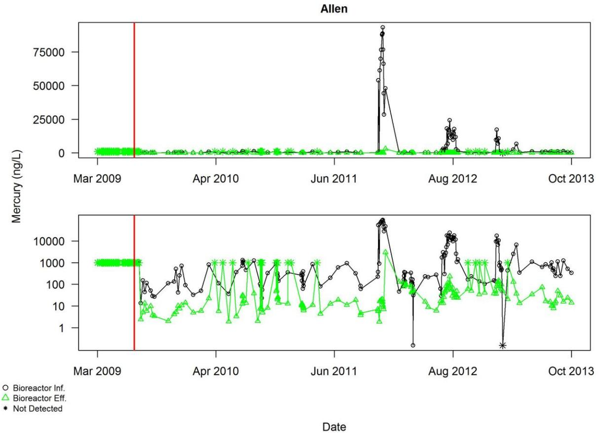
Figure A4.5.6 Bioreactor effluent data of mercury for Allen, prior to excluding any data for reasons described in Section 3.2. Pollutant concentrations are shown on a linear scale in the upper plot, log scale in the lower plot. The red vertical line indicates the end of the commissioning period
