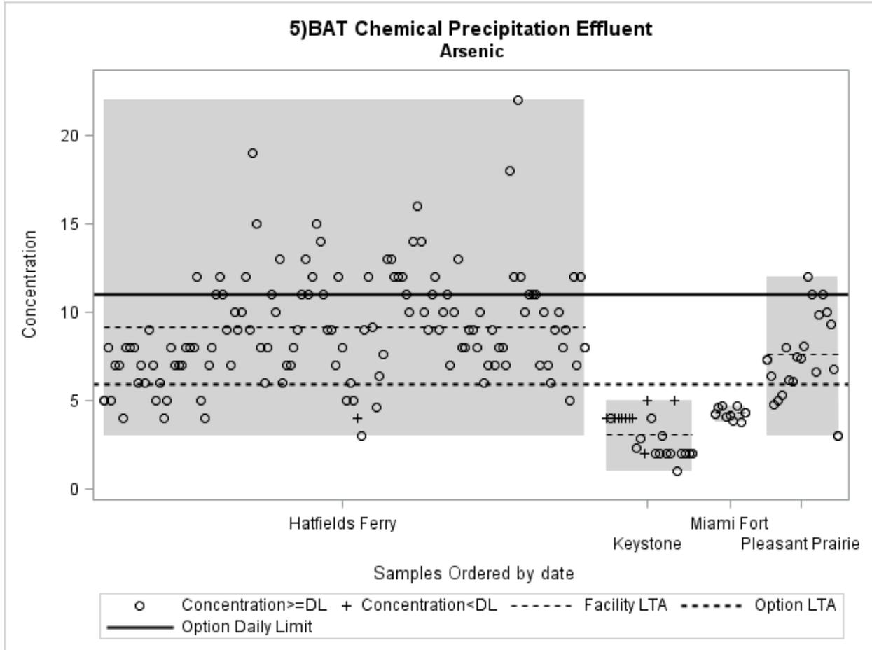
Figure A7.2 Arsenic daily limitation and daily concentrations ( $\mu\text{g/L}$ ) at Hatfield's Ferry used to calculate the limitations based on chemical precipitation treatment of FGD wastewater
