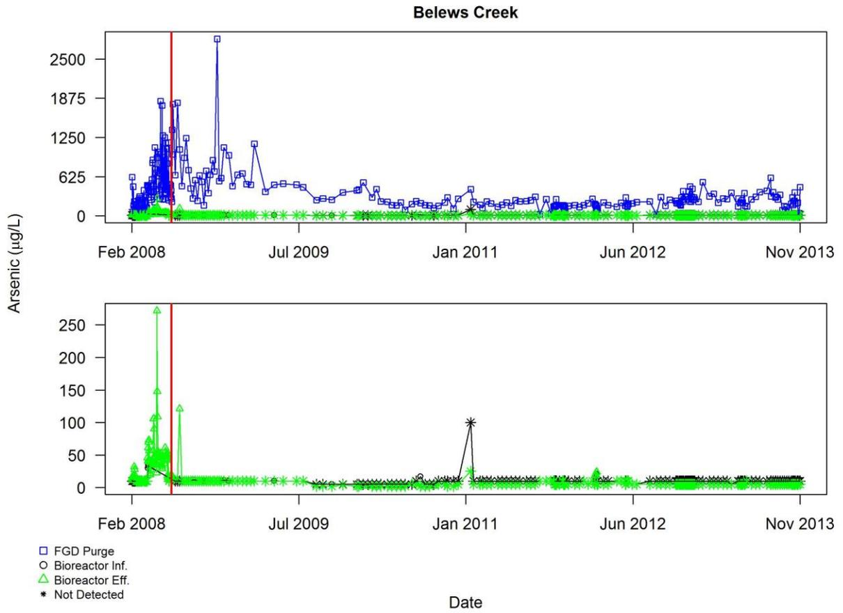
Figure A3.2.4 Plot of self-monitoring data for arsenic ( $\mu\text{g/L}$ ) for Belews Creek after exclusions other than commissioning period described in Section 3.2 and superimposed with smooth curves using LOWESS. The red vertical line indicates the end of the commissioning period
