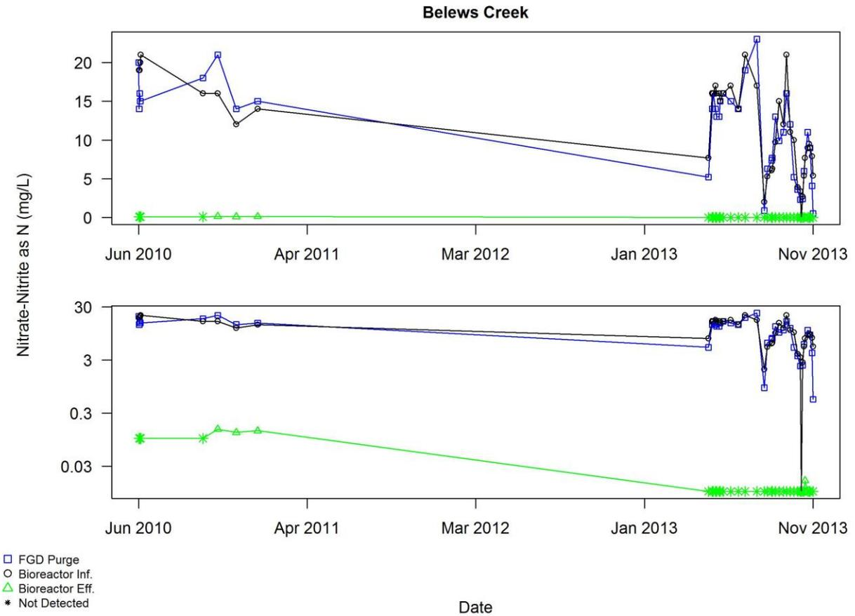
**Figure A4.6.8 Bioreactor influent and Bioreactor effluent data of Nitrate-Nitrite as N for Belews Creek, prior to excluding any data for reasons described in Section 3.2. Pollutant concentrations are shown on a linear scale in the upper plot, log scale in the lower plot**
