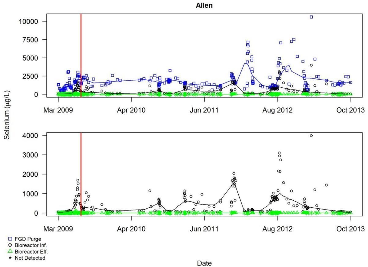
Figure A3.1.17 Plot of all self-monitoring data for selenium ( $\mu\text{g/L}$ ) for Allen, bioreactor effluent only. The red vertical line indicates the end of the commissioning period
