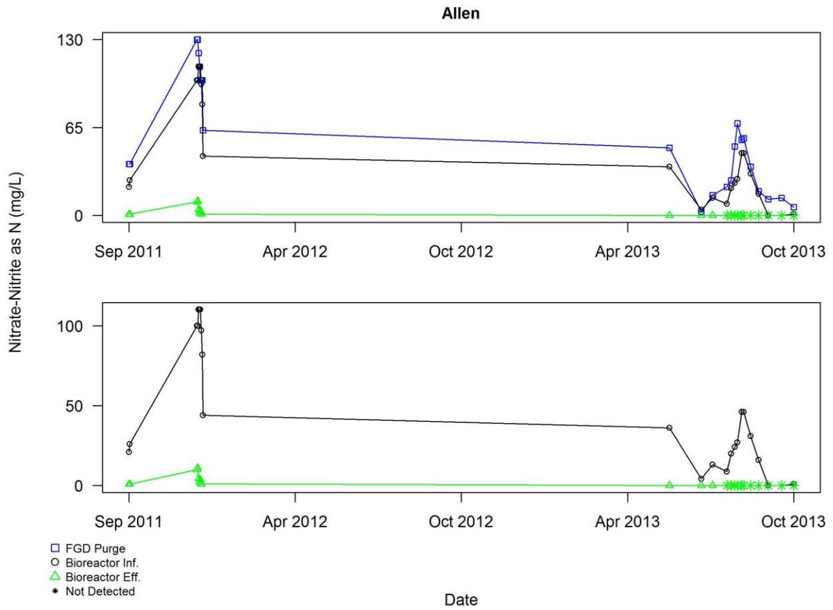
Figure A3.1.10 Plot of all self-monitoring data for Nitrate-Nitrite as N (mg/L) for Allen superimposed with smooth curves using LOWESS
