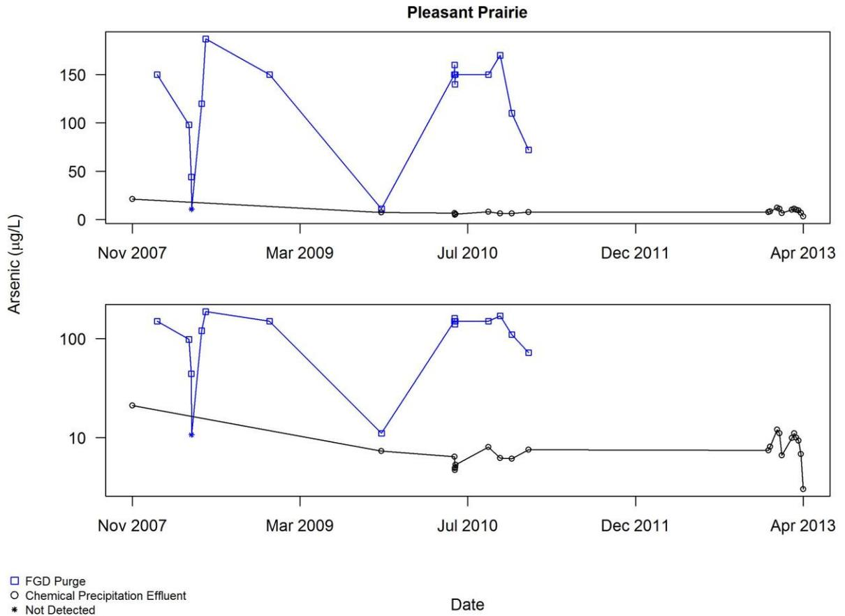
**Figure A4.4.2 Chemical precipitation effluent data of arsenic for Pleasant Prairie, prior to excluding any data for reasons described in Section 3.2. Pollutant concentrations are shown on a linear scale in the upper plot, log scale in the lower plot**
