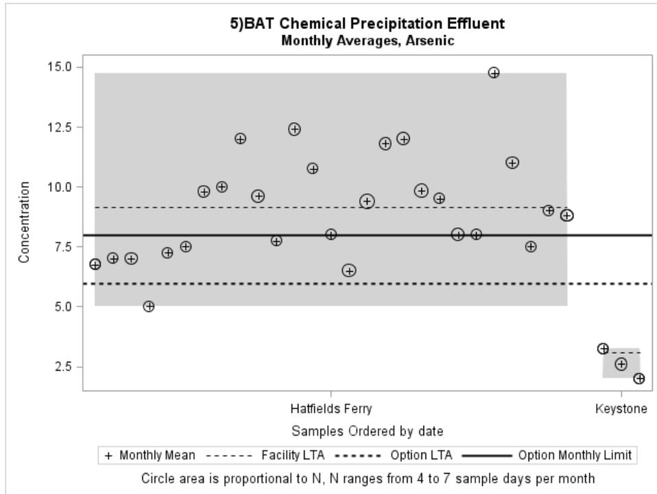
**Figure A7.12 Arsenic monthly limitation and monthly average concentrations ( $\mu\text{g/L}$ ) at Hatfield's Ferry for chemical precipitation treatment of FGD wastewater**
