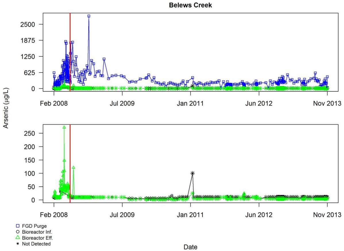
Figure A3.2.2 Plot of all self-monitoring data for arsenic ( $\mu\text{g/L}$ ) for Belews Creek superimposed with smooth curves using LOWESS. The red vertical line indicates the end of the commissioning period
