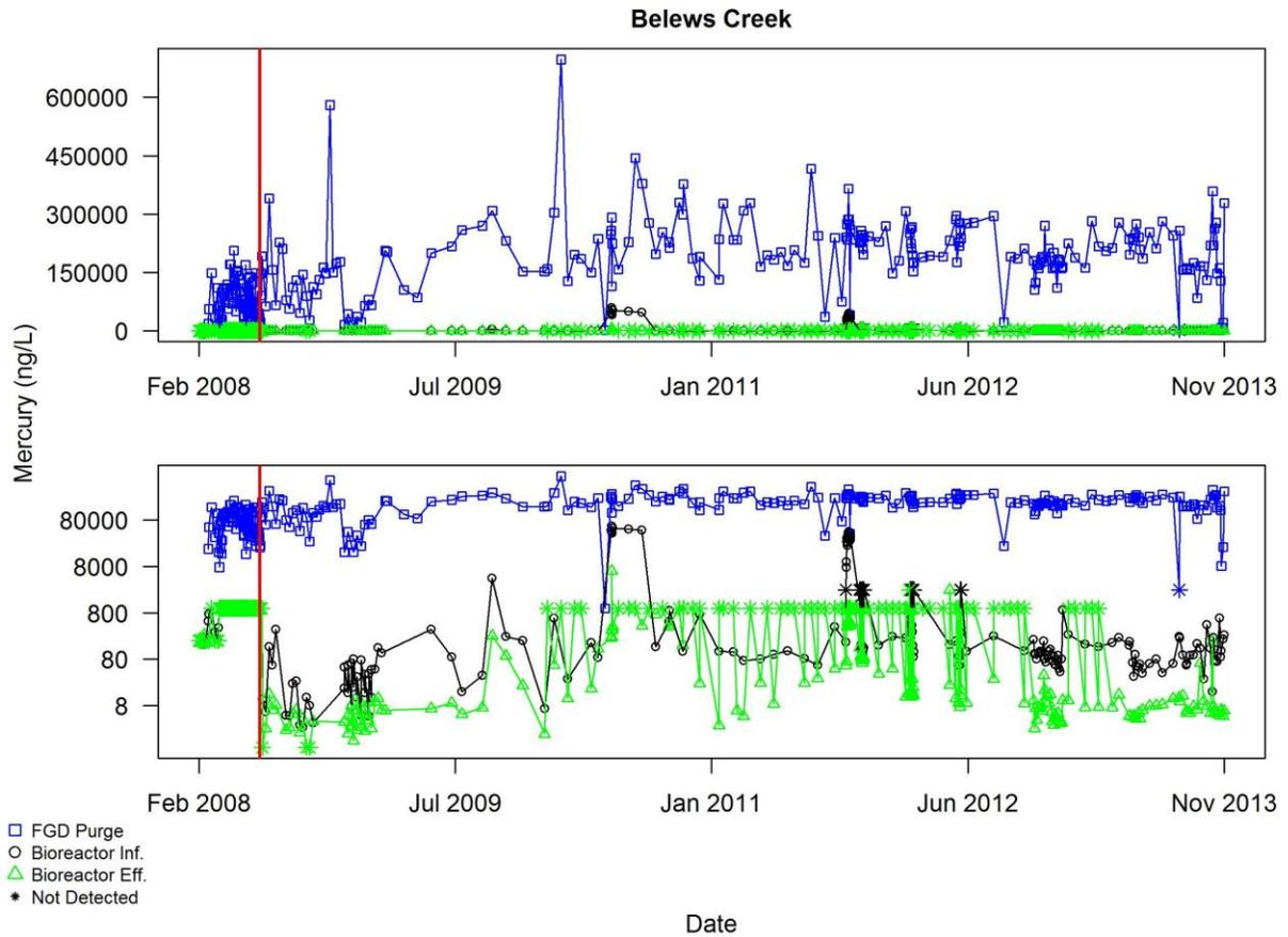
**Figure A4.6.5** Bioreactor influent and Bioreactor effluent data of mercury for Belews Creek, prior to excluding any data for reasons described in Section 3.2. Pollutant concentrations are shown on a linear scale in the upper plot, log scale in the lower plot. The red vertical line indicates the end of the commissioning period
