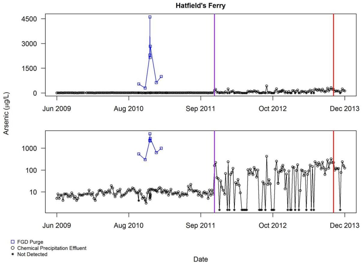
**Figure A4.1.2 Chemical precipitation effluent data of arsenic for Hatfield's Ferry, prior to excluding any data for reasons described in Section 3.2. Pollutant concentrations are shown on a linear scale in the upper plot, log scale in the lower plot. The purple vertical line indicates the point when the plant changed analytical laboratories, and the red vertical line indicates the start of decommissioning period**
