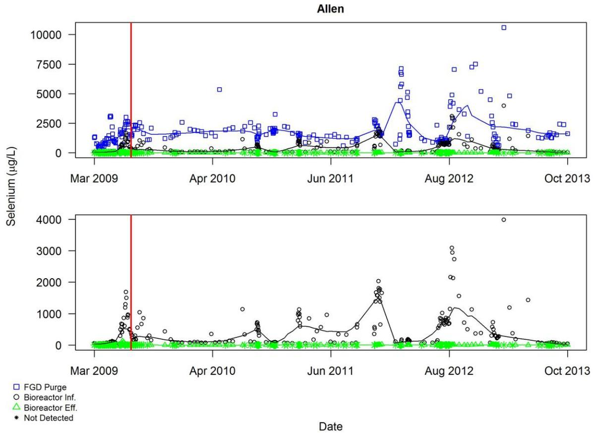
Figure A3.1.15 Plot of self-monitoring data for selenium ( $\mu\text{g/L}$ ) for Allen after exclusions other than commissioning period described in Section 3.2. The red vertical line indicates the end of the commissioning period
