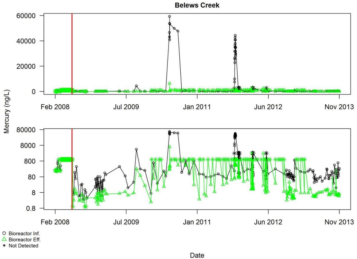
**Figure A4.6.6** Bioreactor effluent data of mercury for Belews Creek, prior to excluding any data for reasons described in Section 3.2. Pollutant concentrations are shown on a linear scale in the upper plot log scale in the lower plot. The red vertical line indicates the end of the commissioning period
