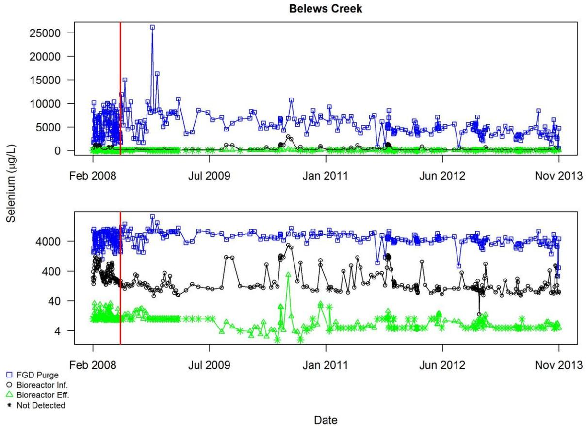
Figure A4.6.11 Bioreactor influent and Bioreactor effluent data of selenium for Belews Creek, prior to excluding any data for reasons described in Section 3.2. Pollutant concentrations are shown on a linear scale in the upper plot, log scale in the lower plot. The red vertical line indicates the end of the commissioning period
