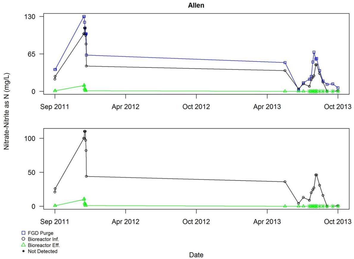
Figure A3.1.12 Plot of self-monitoring data for Nitrate-Nitrite as N (mg/L) for Allen after exclusions other than commissioning period described in Section 3.2 and superimposed with smooth curves using LOWESS
