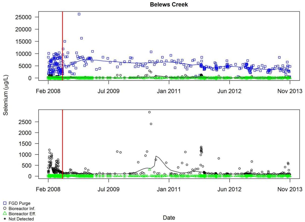
Figure A3.2.15 Plot of self-monitoring data for selenium ( $\mu\text{g/L}$ ) for Belews Creek after exclusions other than commissioning period described in Section 3.2. The red vertical line indicates the end of the commissioning period
