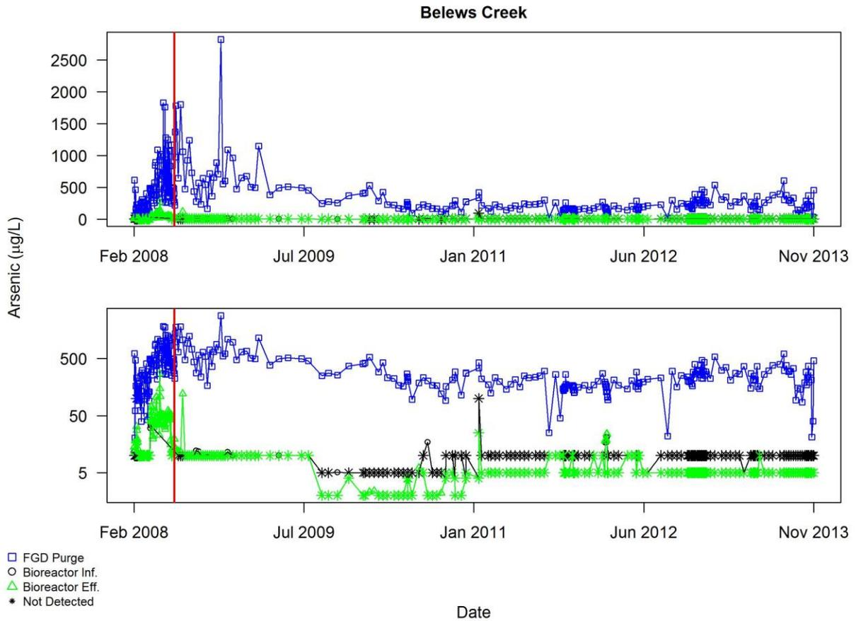
**Figure A4.6.2 Bioreactor influent and Bioreactor effluent data of arsenic for Belews Creek, prior to excluding any data for reasons described in Section 3.2. Pollutant concentrations are shown on a linear scale in the upper plot, log scale in the lower plot. The red vertical line indicates the end of the commissioning period**
