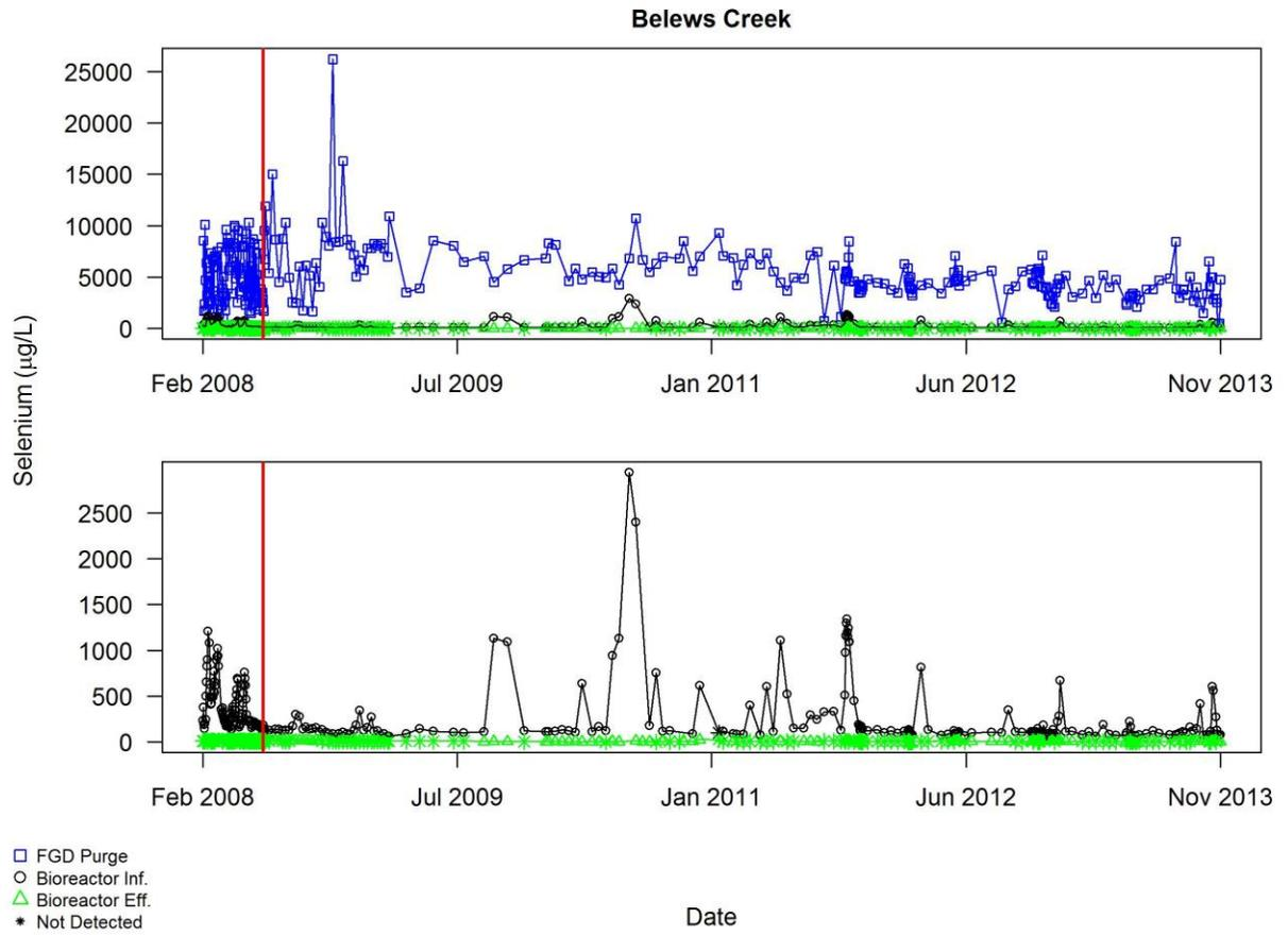
Figure A3.2.16 Plot of self-monitoring data for selenium ( $\mu\text{g/L}$ ) for Belews Creek after exclusions other than commissioning period described in Section 3.2 and superimposed with smooth curves using LOWESS. The red vertical line indicates the end of the commissioning period
