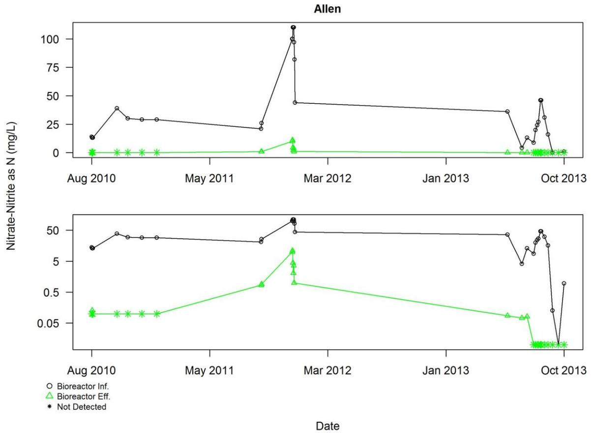
Figure A4.5.9 Bioreactor effluent data of Nitrate-Nitrite as N for Allen, prior to excluding any data for reasons described in Section 3.2. Pollutant concentrations are shown on a linear scale in the upper plot, log scale in the lower plot
