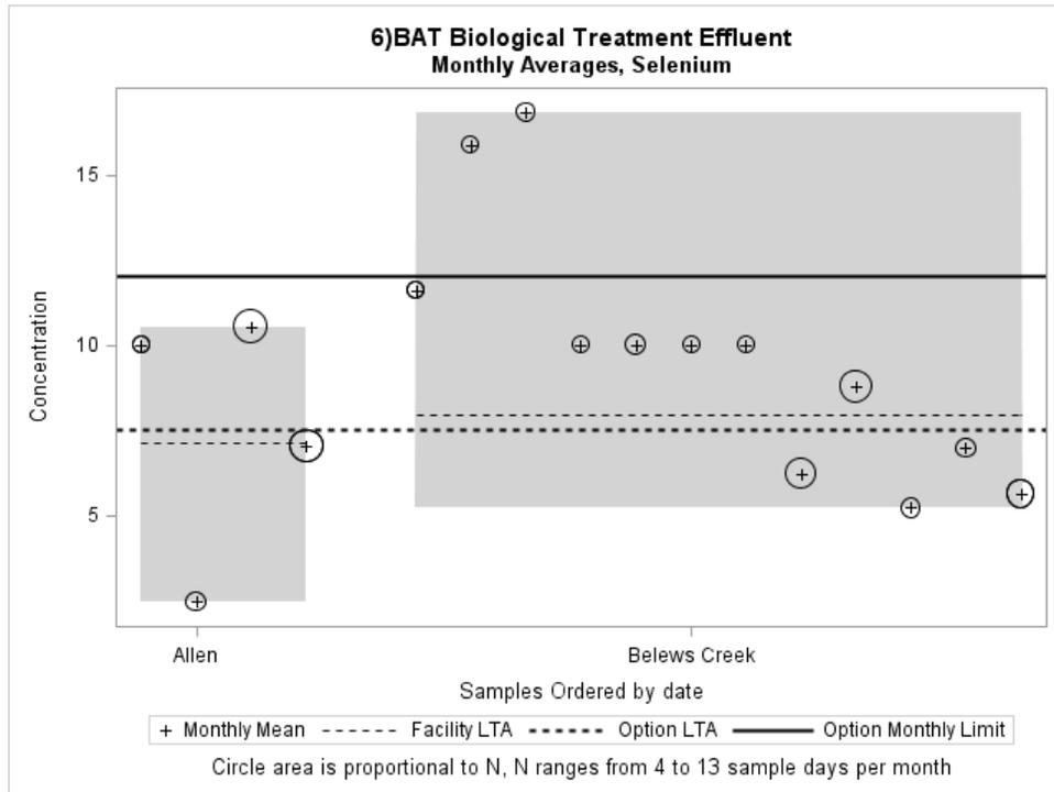
**Figure A7.25 Selenium monthly limitation and monthly average concentrations ( $\mu\text{g/L}$ ) at Allen for biological treatment of FGD wastewater**
