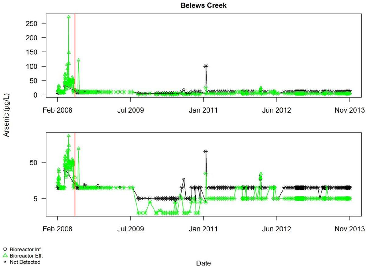
Figure A4.6.3 Bioreactor effluent data of arsenic for Belews Creek, prior to excluding any data for reasons described in Section 3.2. Pollutant concentrations are shown on a linear scale in the upper plot, log scale in the lower plot. The red vertical line indicates the end of the commissioning period
