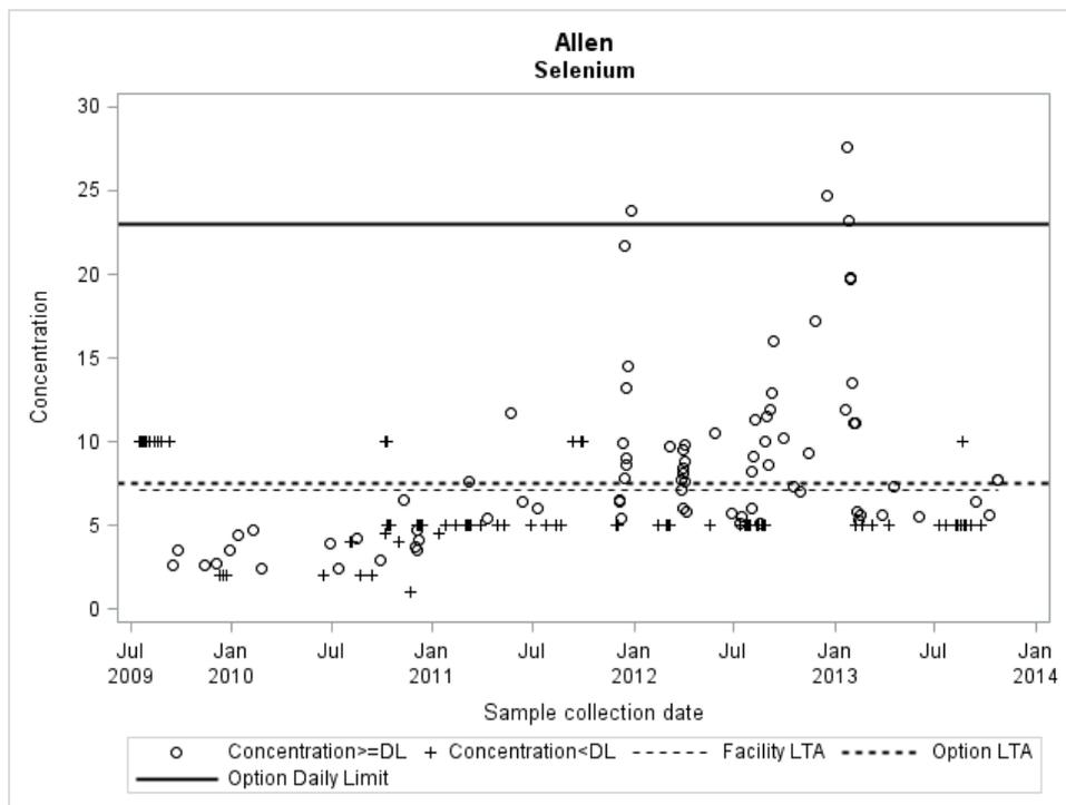
**Figure A7.22 Selenium daily limitation and daily concentrations ( $\mu\text{g/L}$ ) at Belews Creek used to calculate the limitations for biological treatment of FGD wastewater**
