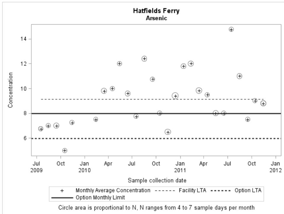
**Figure A7.13** Arsenic monthly limitation and monthly average concentrations ( $\mu\text{g/L}$ ) at Keystone for chemical precipitation treatment of FGD wastewater
