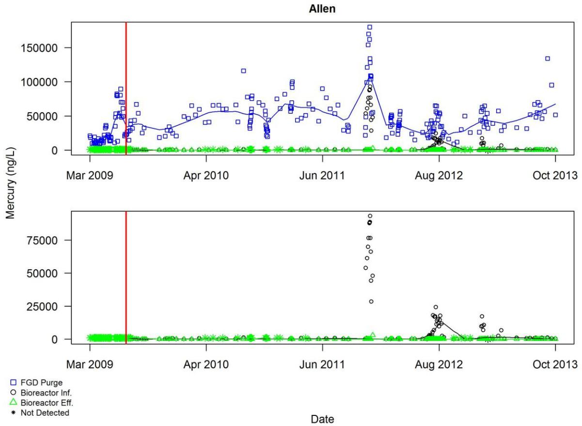
Figure A3.1.7 Plot of self-monitoring data for mercury (ng/L) for Allen after exclusions other than commissioning period described in Section 3.2. The red vertical line indicates the end of the commissioning period
