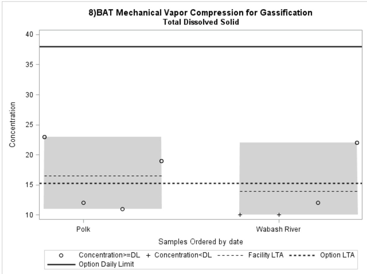
**Figure A7.37** Total dissolved solid daily limitation and daily concentrations (mg/L) at Polk used to calculate the limitations for the vapor-compression evaporation treatment technology option for gasification wastewater
