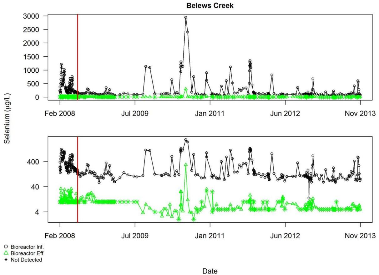
Figure A4.6.12 Bioreactor effluent data of selenium for Belews Creek, prior to excluding any data for reasons described in Section 3.2. Pollutant concentrations are shown on a linear scale in the upper plot, log scale in the lower plot. The red vertical line indicates the end of the commissioning period
