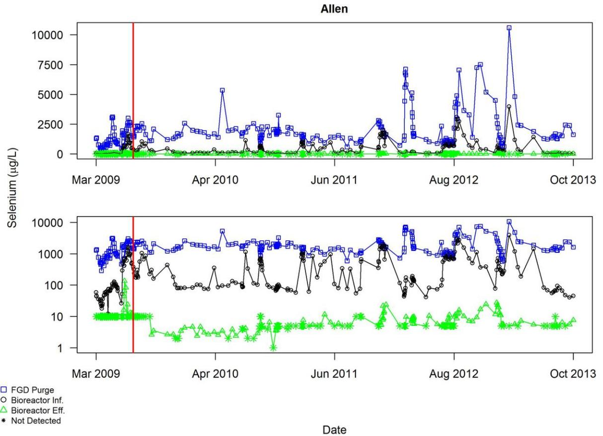
**Figure A4.5.11 Bioreactor influent and Bioreactor effluent data of selenium for Allen, prior to excluding any data for reasons described in Section 3.2. Pollutant concentrations are shown on a linear scale in the upper plot, log scale in the lower plot. The red vertical line indicates the end of the commissioning period**
