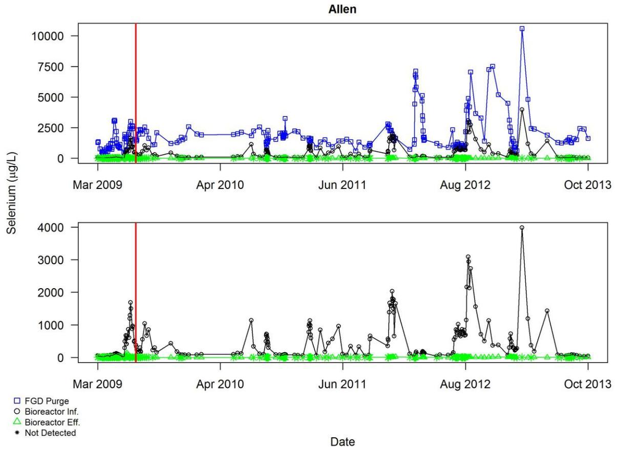
Figure A3.1.16 Plot of self-monitoring data for selenium ( $\mu\text{g/L}$ ) for Allen after exclusions other than commissioning period described in Section 3.2 and superimposed with smooth curves using LOWESS. The red vertical line indicates the end of the commissioning period
