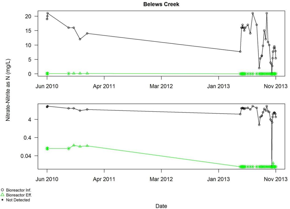
Figure A4.6.9 Bioreactor effluent data of Nitrate-Nitrite as N for Belews Creek, prior to excluding any data for reasons described in Section 3.2. Pollutant concentrations are shown on a linear scale in the upper plot, log scale in the lower plot
