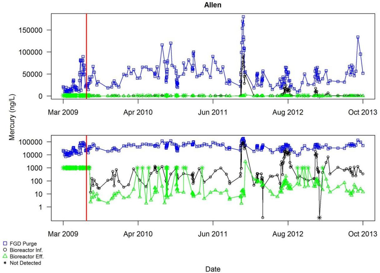
**Figure A4.5.5 Bioreactor influent and Bioreactor effluent data of mercury for Allen, prior to excluding any data for reasons described in Section 3.2. Pollutant concentrations are shown on a linear scale in the upper plot, log scale in the lower plot. The red vertical line indicates the end of the commissioning period**
