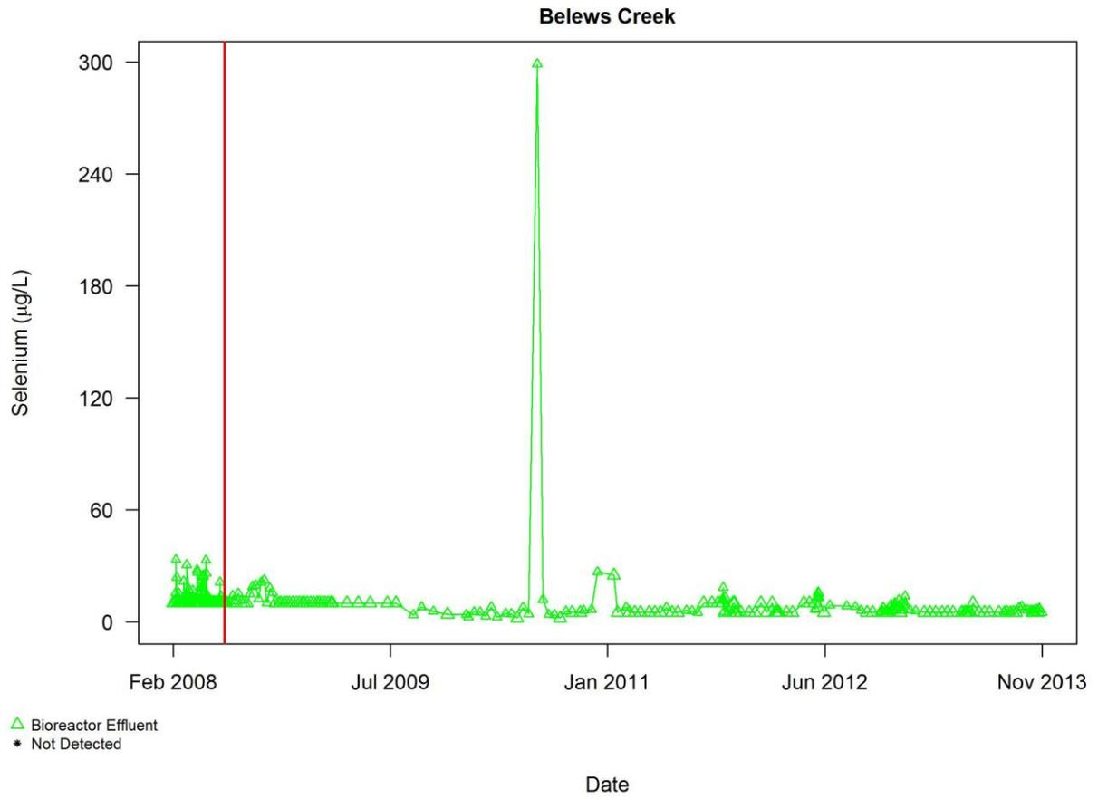
Figure A3.2.18 Plot of all self-monitoring data for selenium ( $\mu\text{g/L}$ ) for Belews Creek superimposed with smooth curves using LOWESS, bioreactor effluent only. The red vertical line indicates the end of the commissioning period
