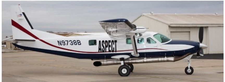
ASPECT consists of a suite of sensors and software mounted in a fixed wing single engine aircraft and uses the principles of remote hazard detection to image, map, identify, and quantify chemical vapors and deposited radioisotopes. It provides first responders – emergency workers on scene -- with actionable information on the situation.
