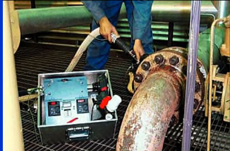
Leak Measurement Using a High Volume Sampler
