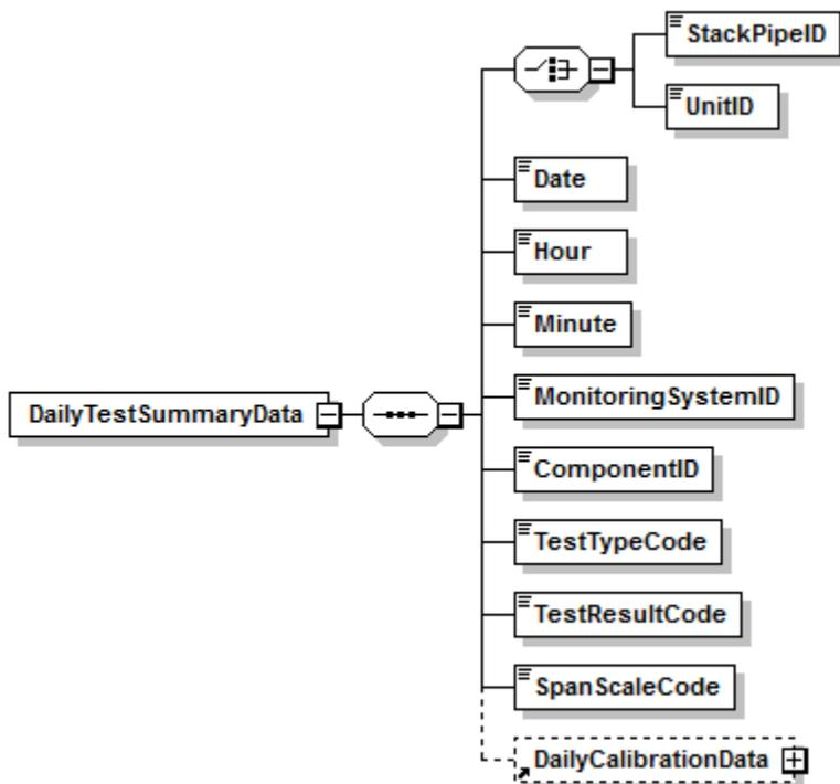
**Daily Test Summary Data XML Elements****Unit ID or Stack Pipe ID** (*UnitID or StackPipeID*)
