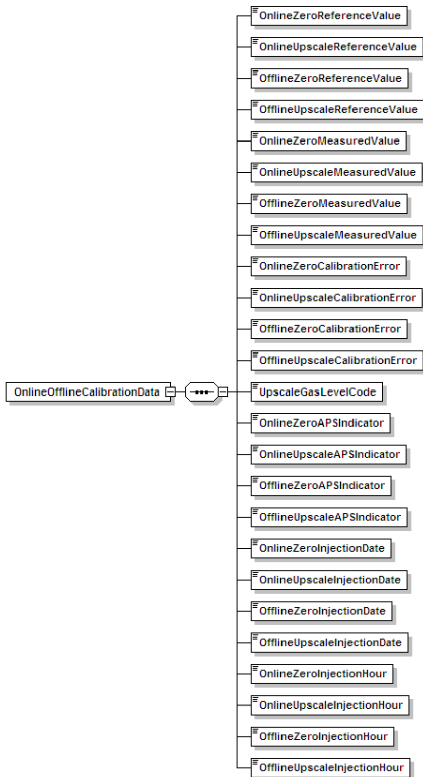
Figure 30: Online Offline Calibration Data XML Elements
