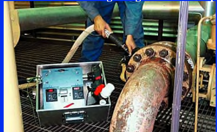
Leak Measurement Using a High Volume Sampler
