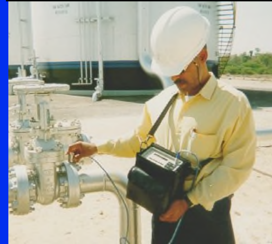
Leak Measurement Using a High Volume Sampler
