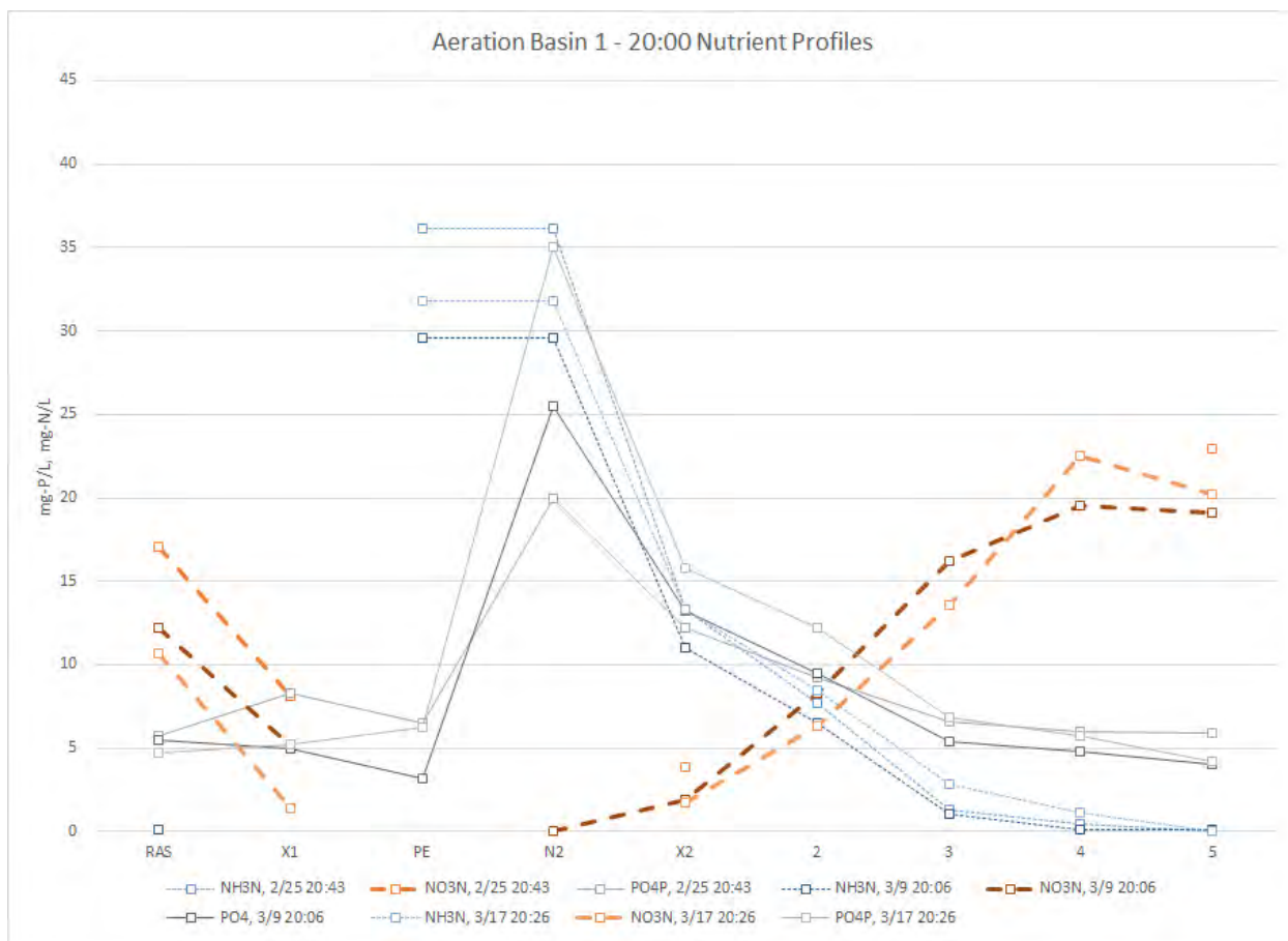
Figure 24. West Boise WWTF – Aeration Basin 1 Nutrient Profile, 20:00 (Average PE = 8.1 MGD, Average RAS = 3.0 MGD)
