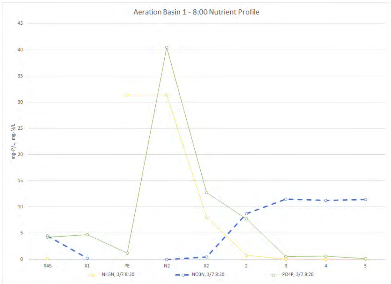
Figure 22. West Boise WWTF – Aeration Basin 1 Nutrient Profile, 8:20 (PE = 5.31 MGD, RAS = 2.22 MGD)
