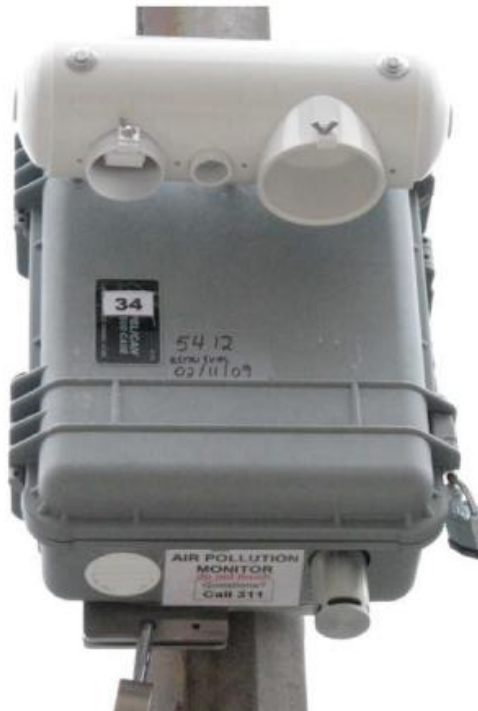
Figure 11.2.1 Integrated Filter-based PM 2.5 Sampling Unit
