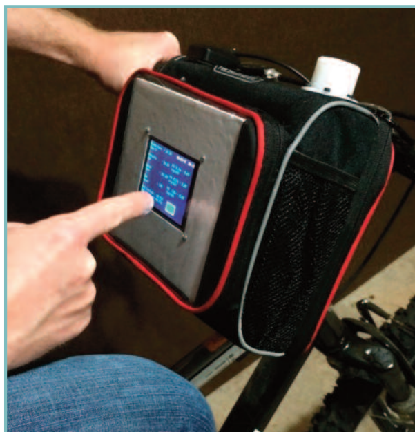
Figure 2. The portable AirMapper with carrying strap and touchscreen.
