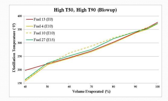
As ethanol content increases in the test fuels, the "T70 bump" also increases.
