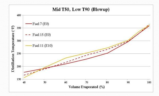
Within every set of EPAct test fuels with matched T50 and T90, and varying ethanol concentrations, the boiling points of one or more higher-ethanol fuels exceeded those of one or more lower-ethanol fuels for the entire T60-T80 range.
