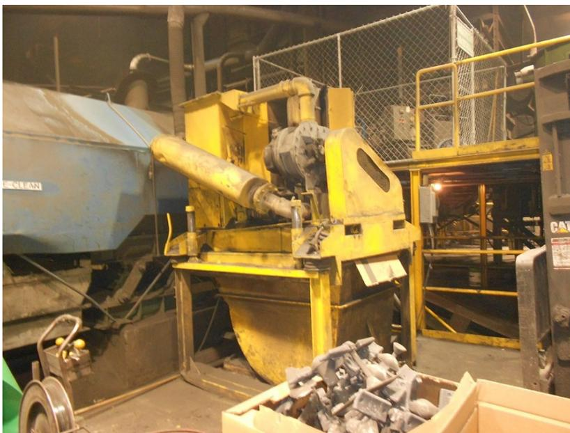
*Industrial vacuum used to remove dry asbestos insulation*
