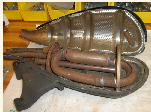
Muffler: cut open
