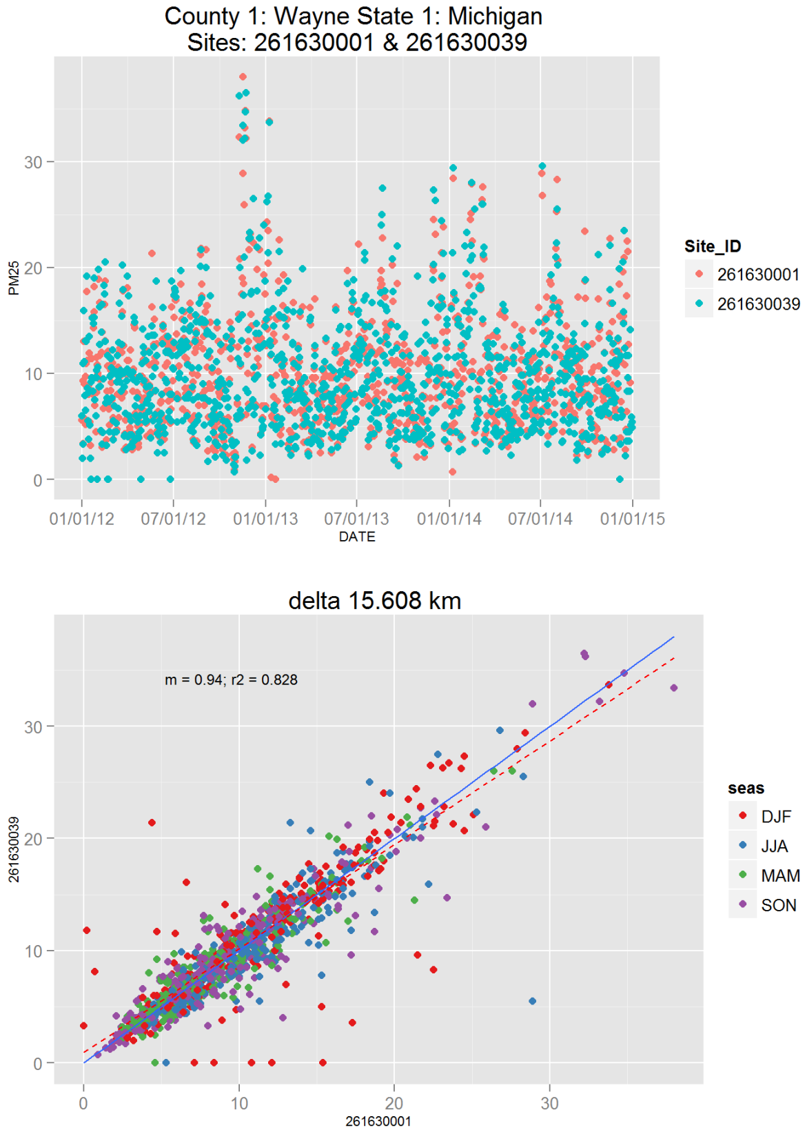
Figure 123: Comparison of PM 2.5 data for sites 261630001 and 261630001. Top panel shows time series for both sites for years 2012-2014. Bottom panel shows scatter plot of paired data, along with slope for the linear regression and correlation coefficient (r 2 ), with data points are colored by month.
