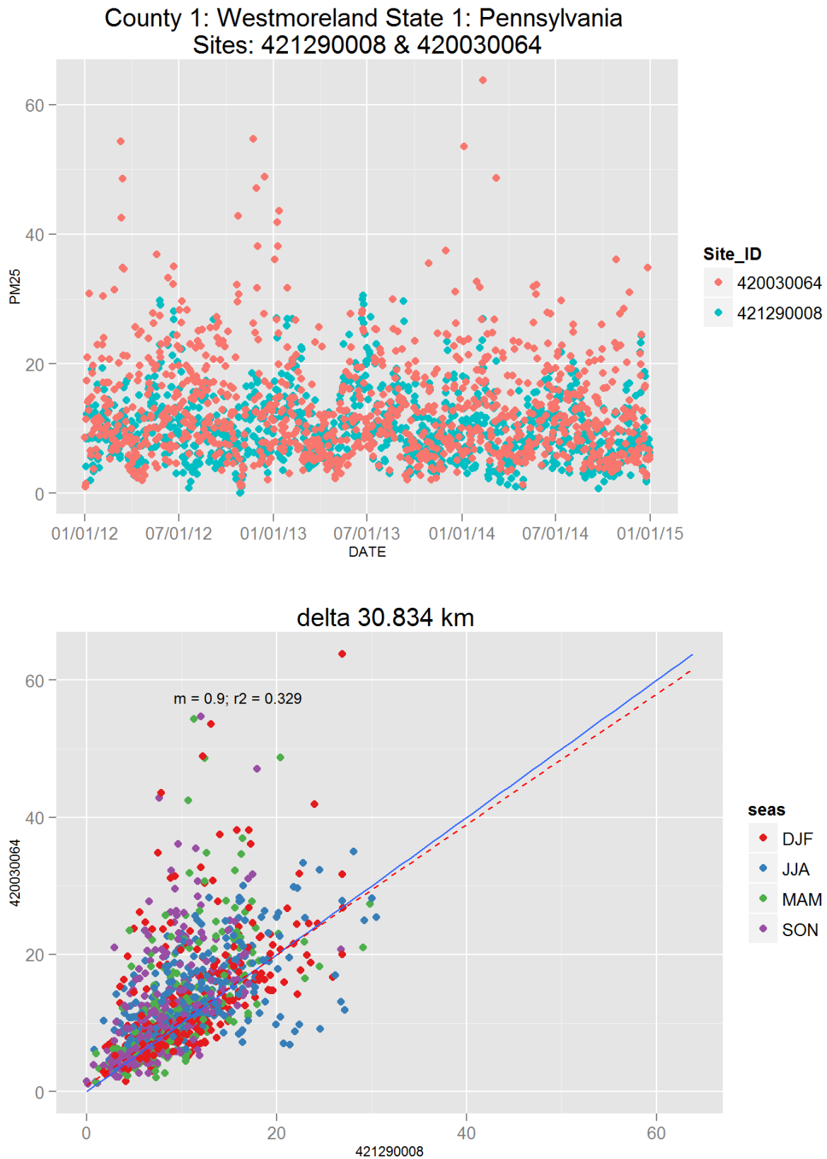
Figure 157: Comparison of PM 2.5 data for sites 421290008 and 420030064. Top panel shows time series for both sites for years 2012-2014. Bottom panel shows scatter plot of paired data, along with slope for the linear regression and correlation coefficient (r 2 ), with data points are colored by month.
