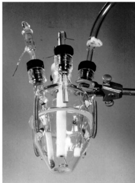
Photograph of a laboratory electroreduction cell for measuring electrical potentials or cyclic voltammetry of electro-reduction reaction (Martin, et al., 2016)
