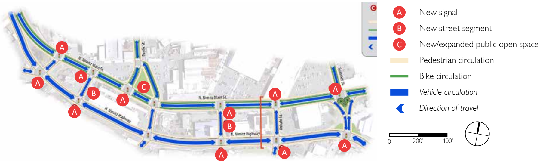
Figure 34. Long-term concept. The addition of vehicle and on-demand pedestrian signals, and narrowed street crossing widths provide a more comfortable and convenient street crossing experience for pedestrians. Adding bike facilities can encourage more people to ride. Separating truck and commute traffic from neighborhood traffic supports a main street character on the mauka side with slower traffic, encouraging more people to walk and linger along the street, as well as enhancing the accessibility and development potential of harbor front parcels.
