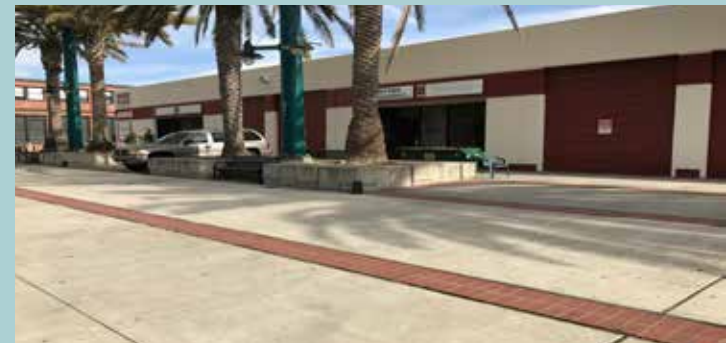
Figure 9. Industrial and commercial uses front onto Park Avenue in Emeryville, CA. The shared street is curbless and uses brick pavers to demark a narrowed drive aisle and parking areas. Raised planters with palms and landscaping define parking, seating, and pedestrian priority spaces.
