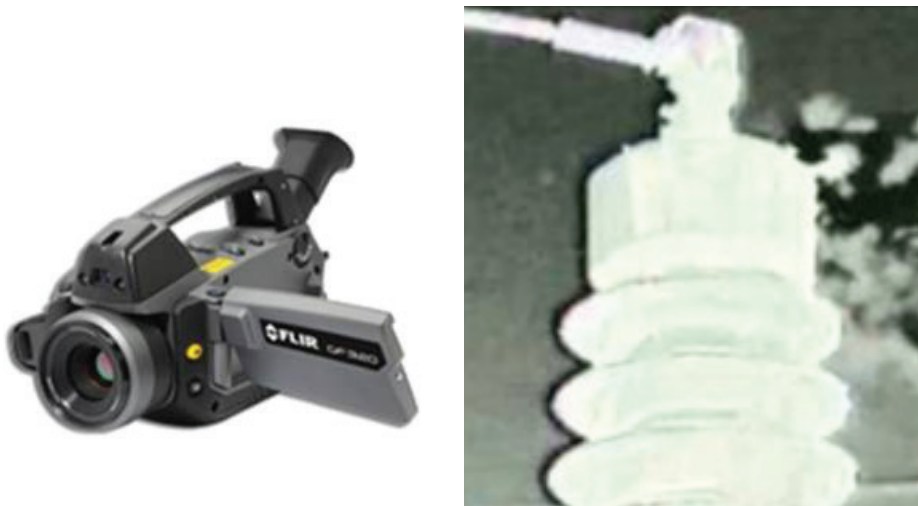
Figure 8. Thermal imaging cameras help visualize the leak of SF 6 . An example camera and an example image captured by the camera are shown above.
