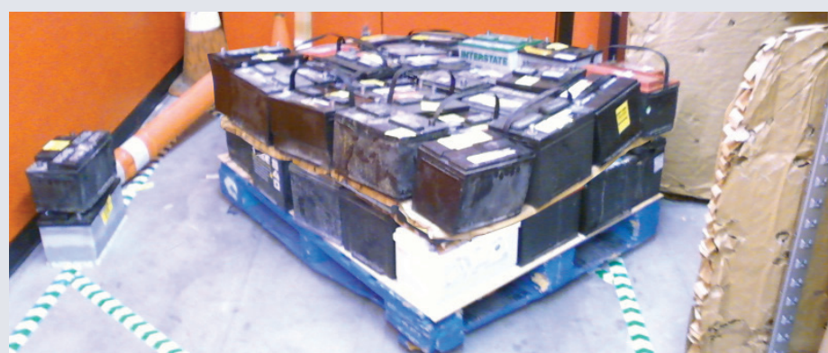
Waste batteries stacked two rows high on pallet.
