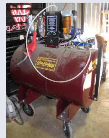
Waste fuel removal pump and containment tank.
