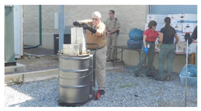
Figure 2: Collected household pharmaceuticals and their packaging being loaded into a burn barrel with a fan.
