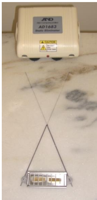
Figure 4. Antistatic Device and ^{210}\text{Po} strip
