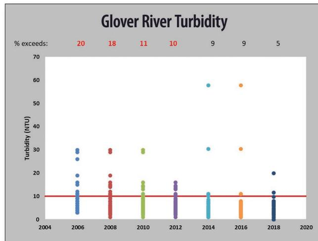
**Figure 2. Turbidity decreased in the Glover River as CPs were installed.**
