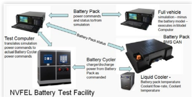
FIGURE 2 Battery Test Setup at EPA NVFEL Battery Test Facility.
