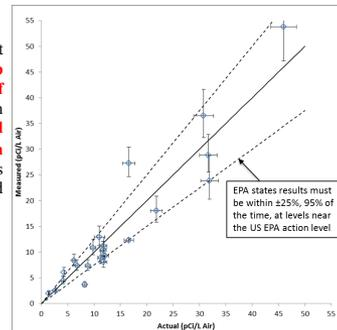
Figure 4. Performance of Radon CTMFD with 1 min sampling times. Results shown with 95% confidence levels.
