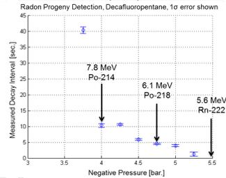
Figure 2. Real-Time, ~95% detection efficiency, alpha spectroscopy with CTMFD system.
