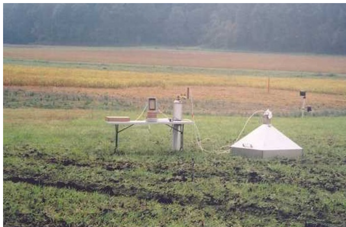
Figure 6-3. Collecting a Flux Sample in the Field
