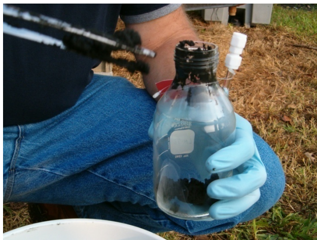
Figure 6-2. Glass Vessel Used for Biosolids Headspace Analysis
