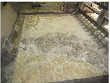
Dissolved Air Flotation Device/a.k.a. "Save All" at APC. This unit reclaims fibers and reuses water during the process. Illegal discharges came from the this unit in the process.
