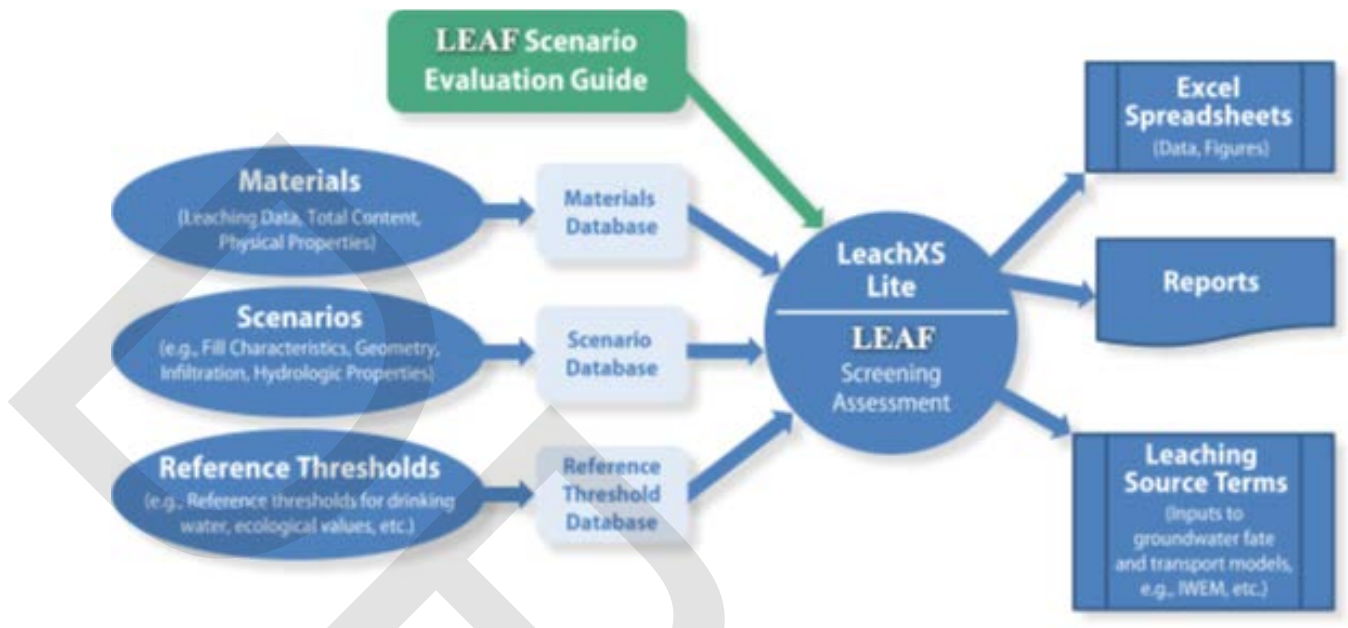
Figure 3-11. LeachXS™ Lite program structure showing data inputs, databases and outputs.
