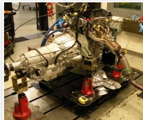
FIGURE 11 Engine and GM 6L80 automatic transmission setup in the test cell.
