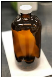
Figure 1: Open-Top Amber Glass Bottle with PTFE-lined Septum
