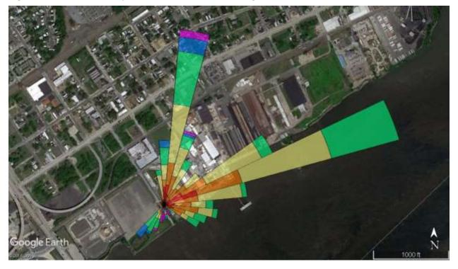
Figure 20. Wind Rose on Days When Silicon Exceeded 0.5 mg/m<sup>3</sup> at the Chester Site
