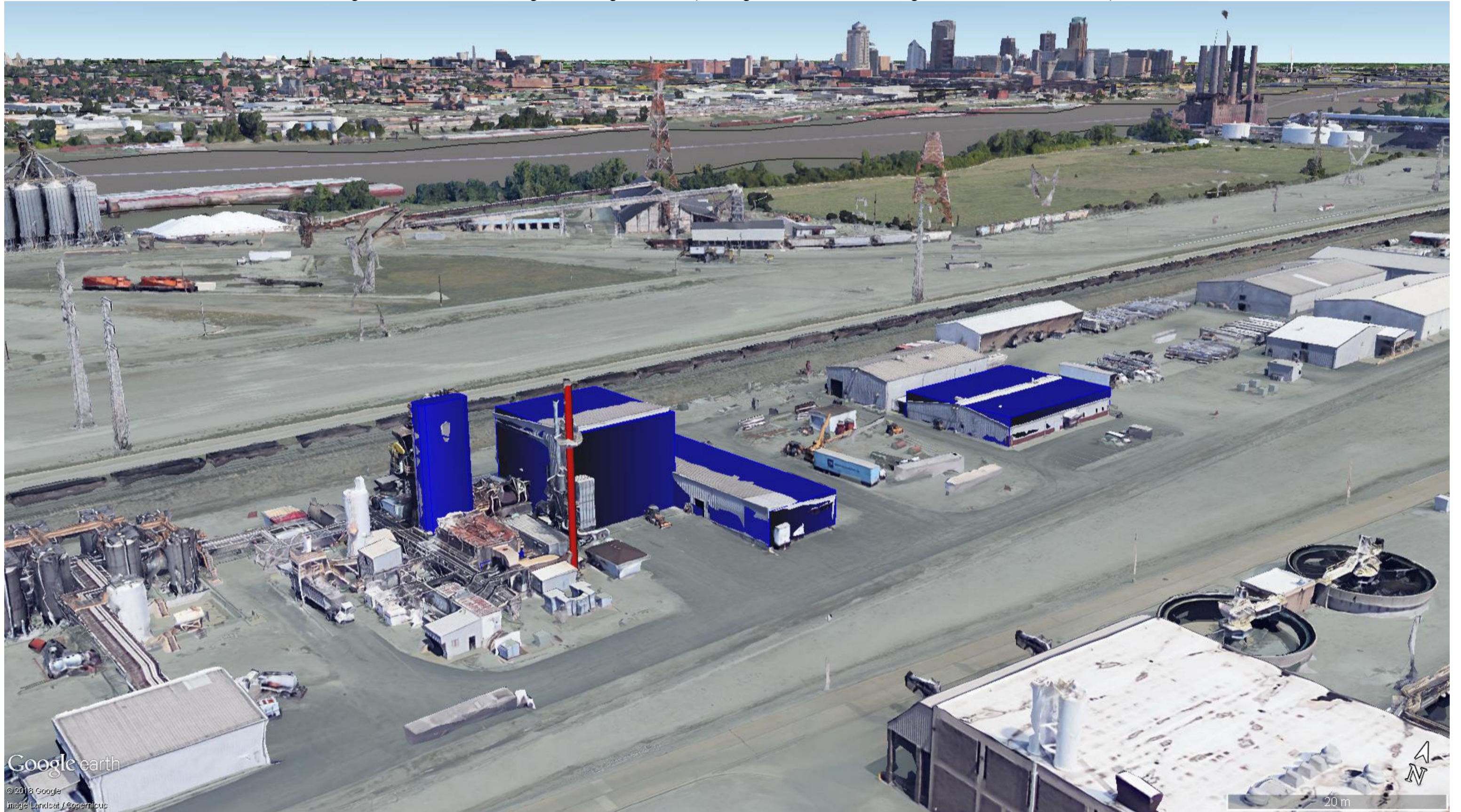
Figure 4-1. 3-Dimensional Image of Buildings and Tanks (Building Downwash Tier 1 Buildings in Blue w/Unit 4 Stack in Red)
