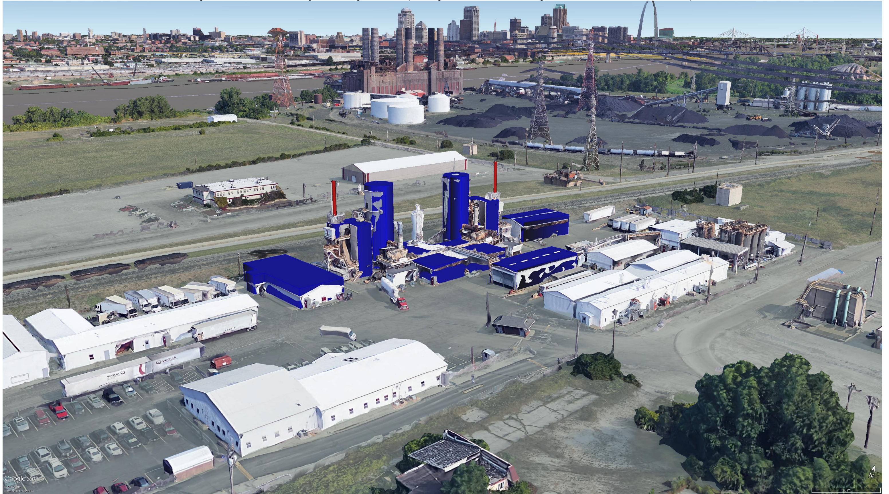
Figure 4-2. 3-Dimensional Image of Buildings and Tanks (Building Downwash Tier 1 Buildings in Blue w/Units 2 and 3 Stacks in Red)
