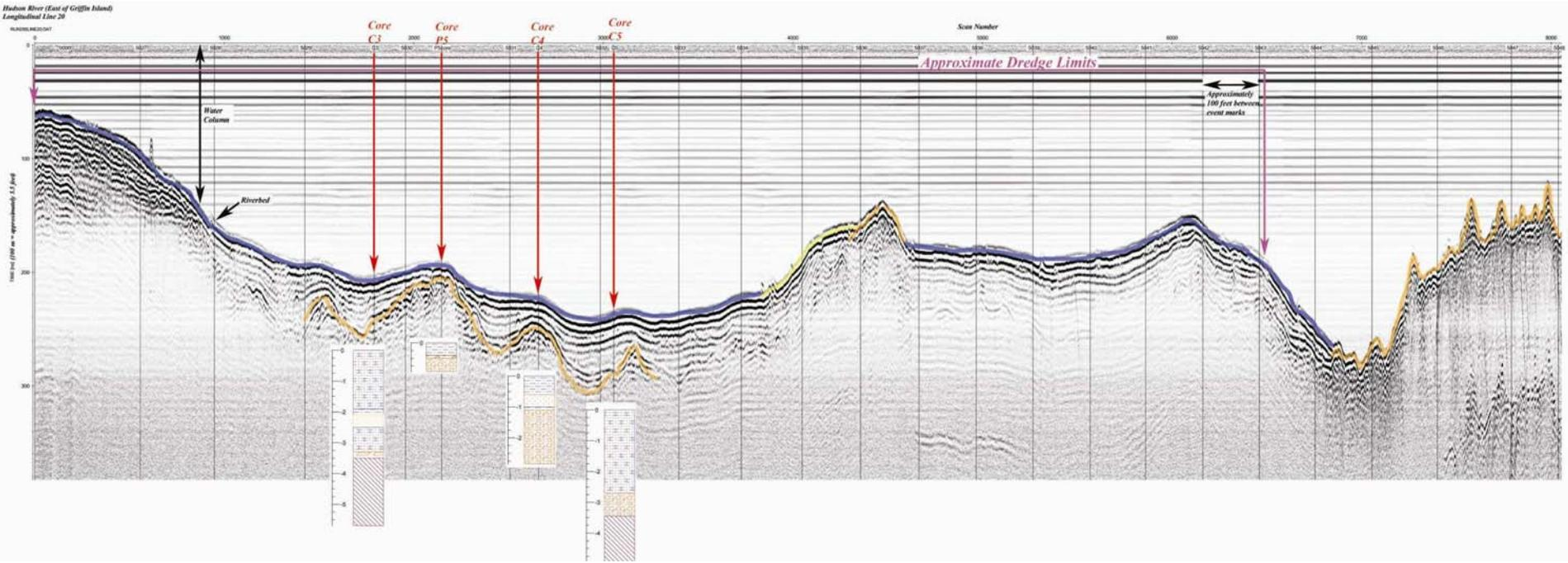
**FIGURE 14** – Reproduced section of GPR data acquired on the east side of Griffin Island. Record provides an example of how ground truth cores were located along a survey line with the primary intent of sampling a specific subbottom reflector (highlighted in orange in this figure). Figure also provides additional illustration of the various GPR classes defined for the project. Note the coarse sediment/rock area identified just outside the proposed dredge limits shown in the figure.
