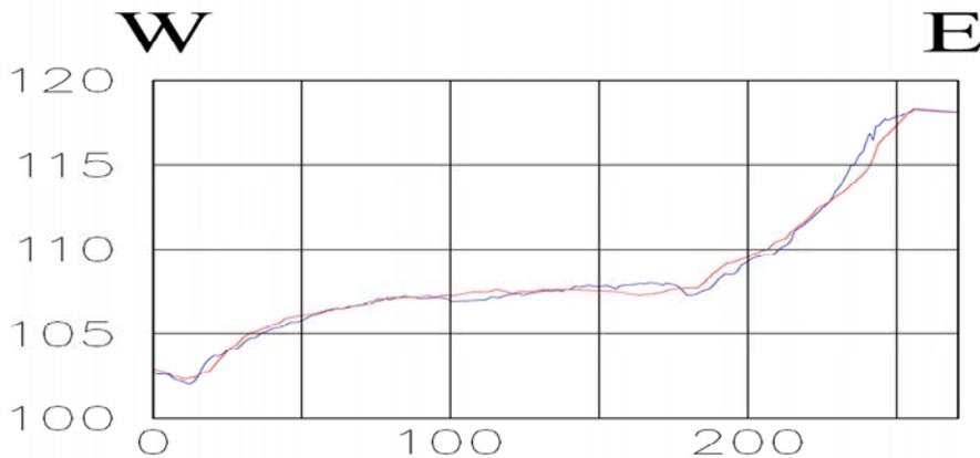
**FIGURE 7** – Representative profile constructed from data acquired in area Main River illustrating where singlebeam and multibeam data match well in the flat areas but differ on the slopes. (Blue line based on multibeam data, red line based on singlebeam data).
