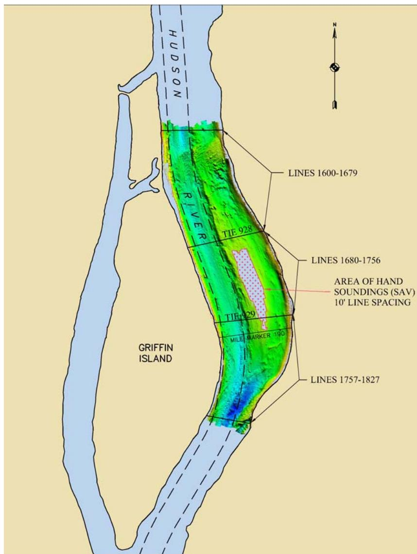
**FIGURE 4** – Multibeam survey coverage in areas adjacent to Griffin Island in River Section 1. Areas with full coverage are represented by a sun-illuminated shaded relief map (blue-green-yellow). Red dots identify areas of SAV where hand soundings were performed. This figure also identifies survey line designations and the sections into which the survey area was subdivided for data processing and QA/QC analysis.
