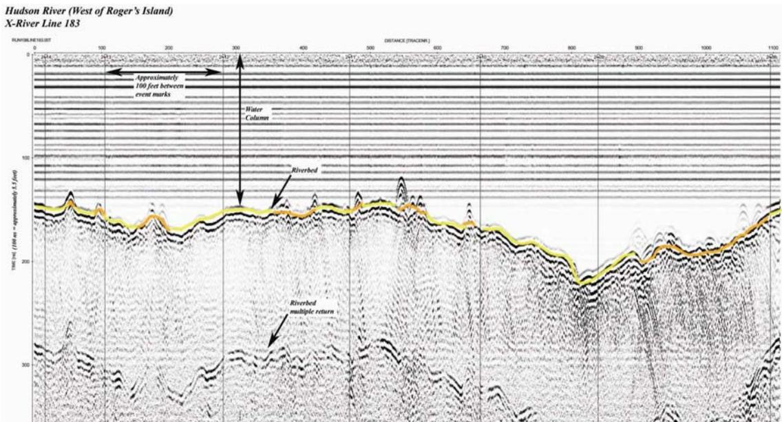
**FIGURE 12** – Reproduced section of GPR data acquired in River Section 1 (west of Rogers Island) which illustrates Class II (orange) and III (yellow) radar reflections. Note the diffraction patterns in the record which indicate the presence of coarse sand, gravel and small rocks in the area.
