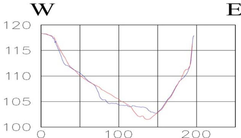
**FIGURE 8** - Representative profile constructed from data acquired in area Rogers Island East illustrating where singlebeam and multibeam data differ in river bed morphology. These differences are interpreted to be associated with erosion and/or sedimentation occurring between the two surveys. (Blue line based on multibeam data, red line based on singlebeam data).
