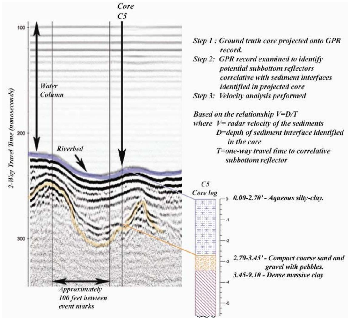
**FIGURE 13** – Reproduced section of GPR data acquired on the east side of Griffin Island which illustrates the process of correlating a specific subbottom reflector to a sediment interface identified in a core.
