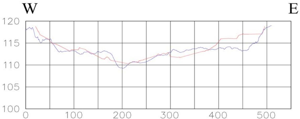
**FIGURE 9** – Representative profile constructed from data acquired in Rogers Island West comparing singlebeam data generated using an interpolated surface and high-density multibeam data. (Blue line based on multibeam data, red line based on singlebeam data).
