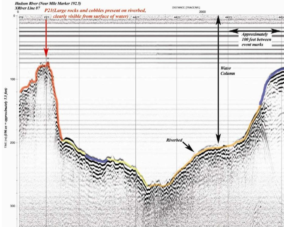
**FIGURE 11** – Reproduced section of GPR data acquired in River Section 1 which illustrates all radar reflective classifications. Radar classes, differentiated by color in the figure correspond to description classifications in Table 5.
