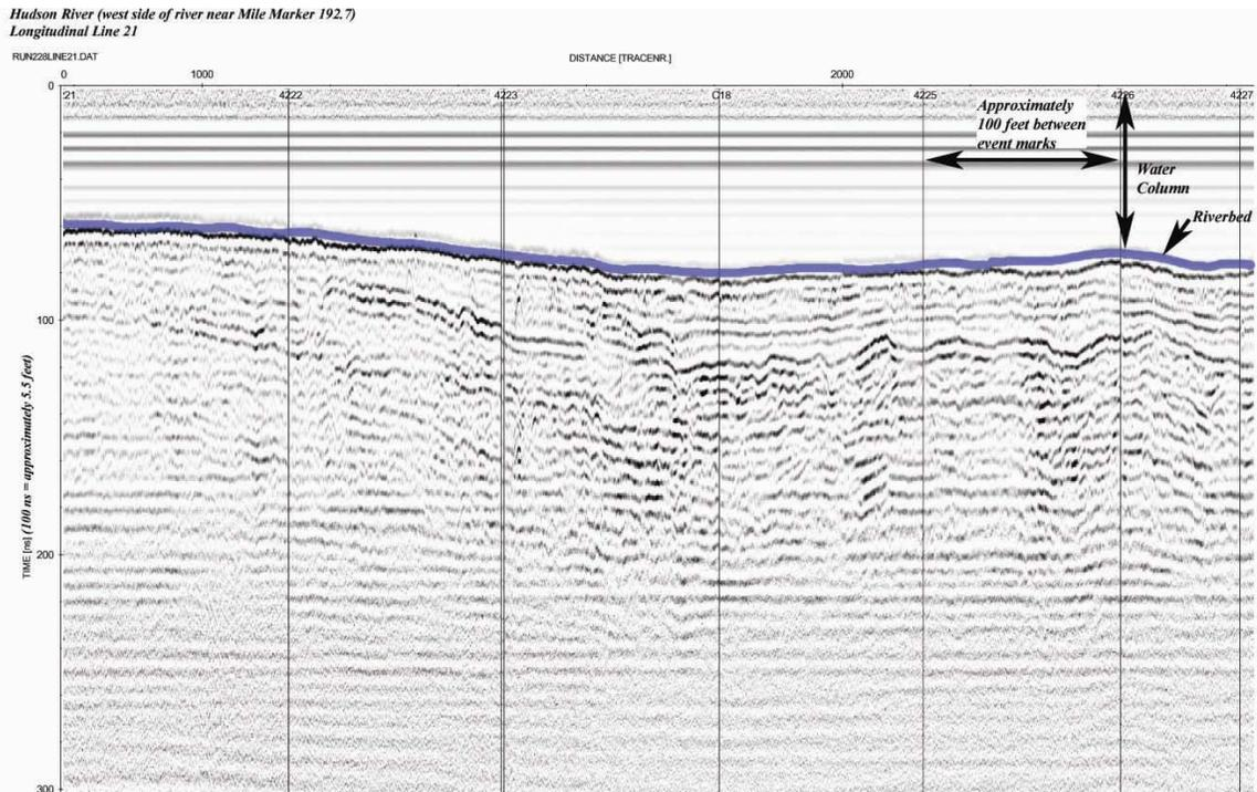
**FIGURE 10** – Reproduced section of GPR data acquired in River Section 1 which exemplifies Class IV radar returns.
