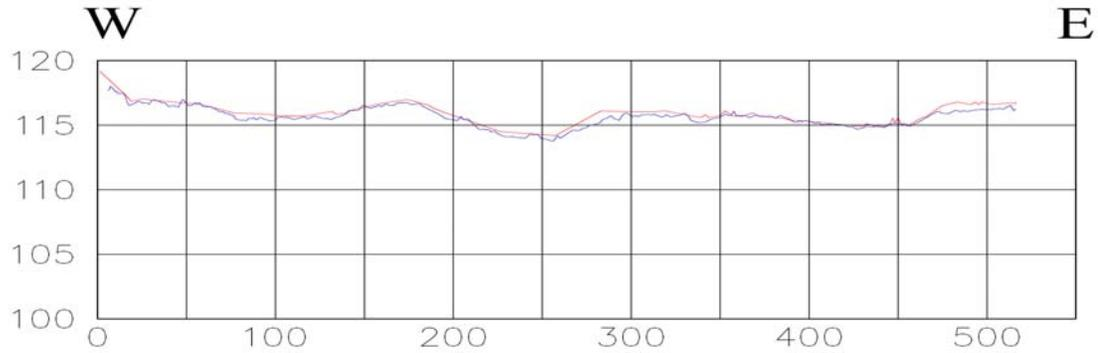
**FIGURE 6** – Representative profile constructed from data acquired in area Rogers Island West illustrating where singlebeam and multibeam data matched well in relatively flat river bed conditions. (Blue line based on multibeam data, red line based on singlebeam data).
