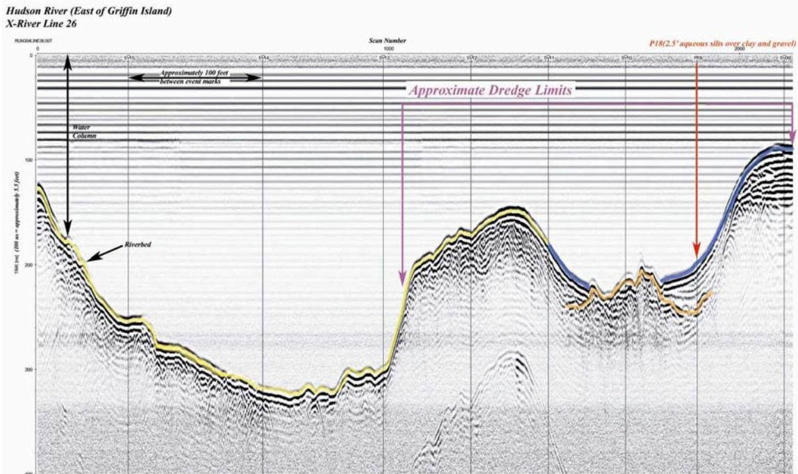
**FIGURE 15** – Reproduced section of GPR data acquired on the east side of Griffin Island. Record identifies a coarse sediment reflector (Class II, highlighted in orange in this figure) cropping out on the river bed within the approximate dredge limits.
