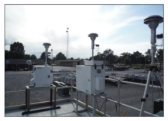
Figure 2: Picture of the intermittent PM<sub>2.5</sub> and PM<sub>10</sub> samplers, as well as the inlet of the PM<sub>2.5</sub> TEOM, on the roof of the Jackson Purchase RECC shelter on October 6, 2014.
