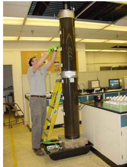
**Figure 2-3. Sediment addition.**
