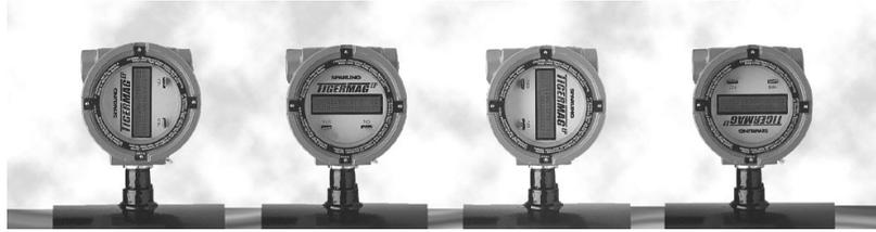
The Sparling TigermagEP's modular display is designed to allow you to rotate the display in four different orientations. The display assembly can be rotated, at 90° intervals, by removing the two screws circled in Figure 3.2 below, for ease of reading the display.
