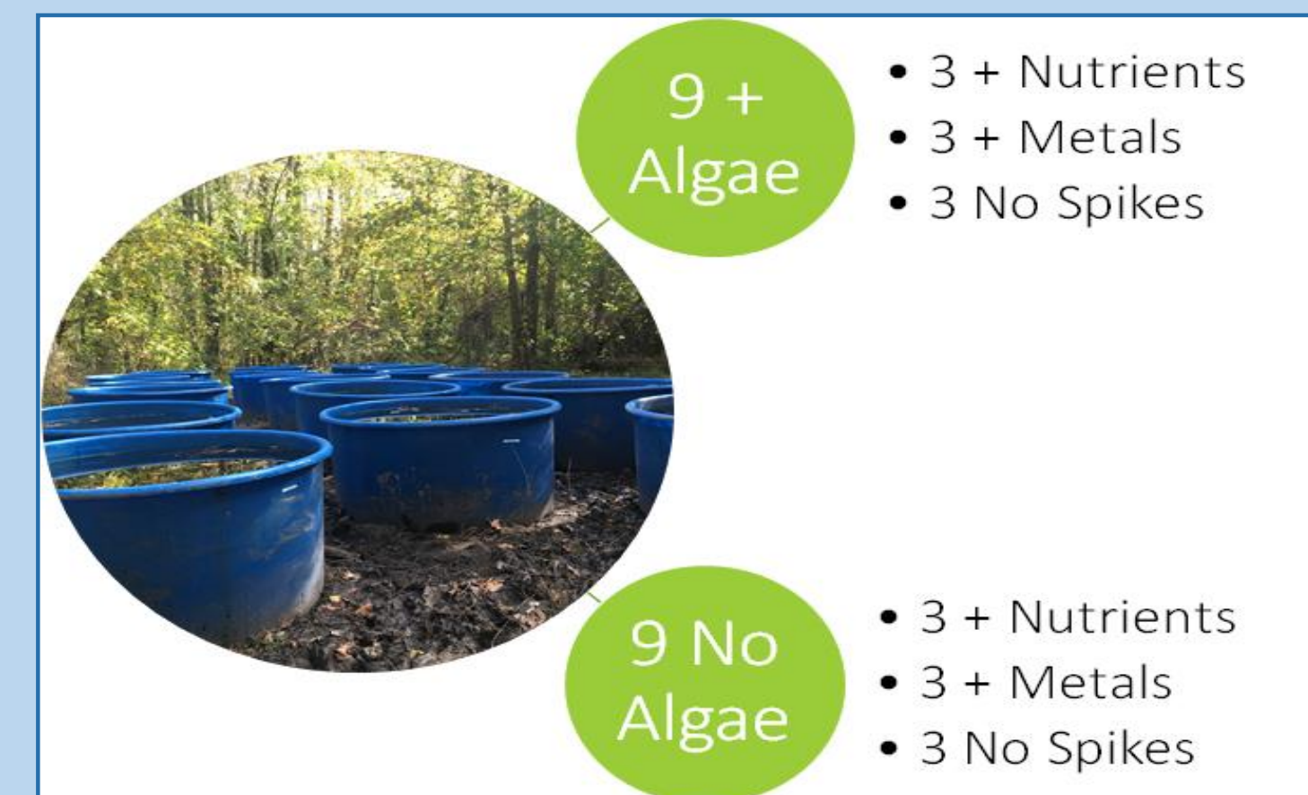
Figure 2. Experimental design for mesocosm experiment: Tanks were filled with lakewater; half received filamentous algae, one third were spiked with nutrients, one third with metals, and one third were not spiked.
