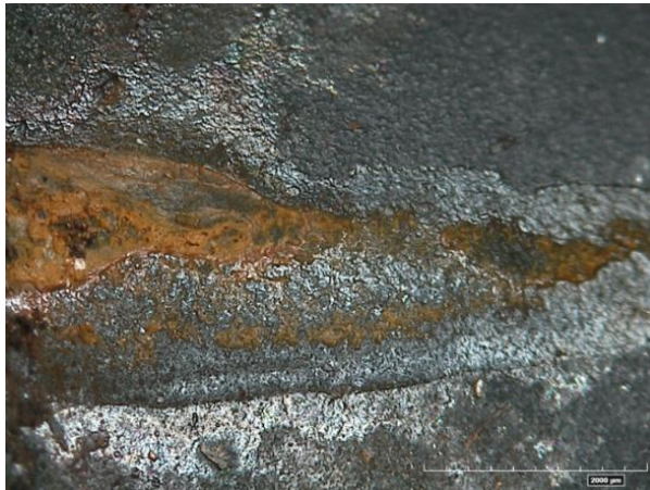
Humid, CsCl: Rusted Gun Barrel
