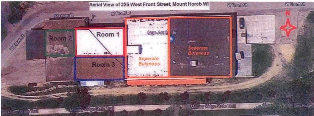
Rooms 1 and 3 are approximately 100 feet (ft.) x 50 ft. and Room 2 is about 50 ft. x 50 ft. The building roof is of wood construction and there is no sprinkler system (i.e. no fire protection).
