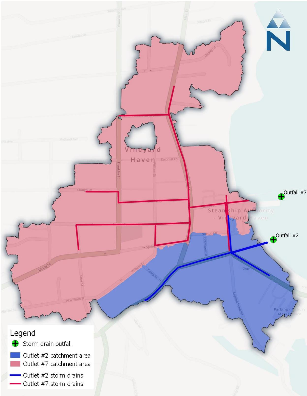
Figure 3. Storm drains, outfalls, and catchment areas
