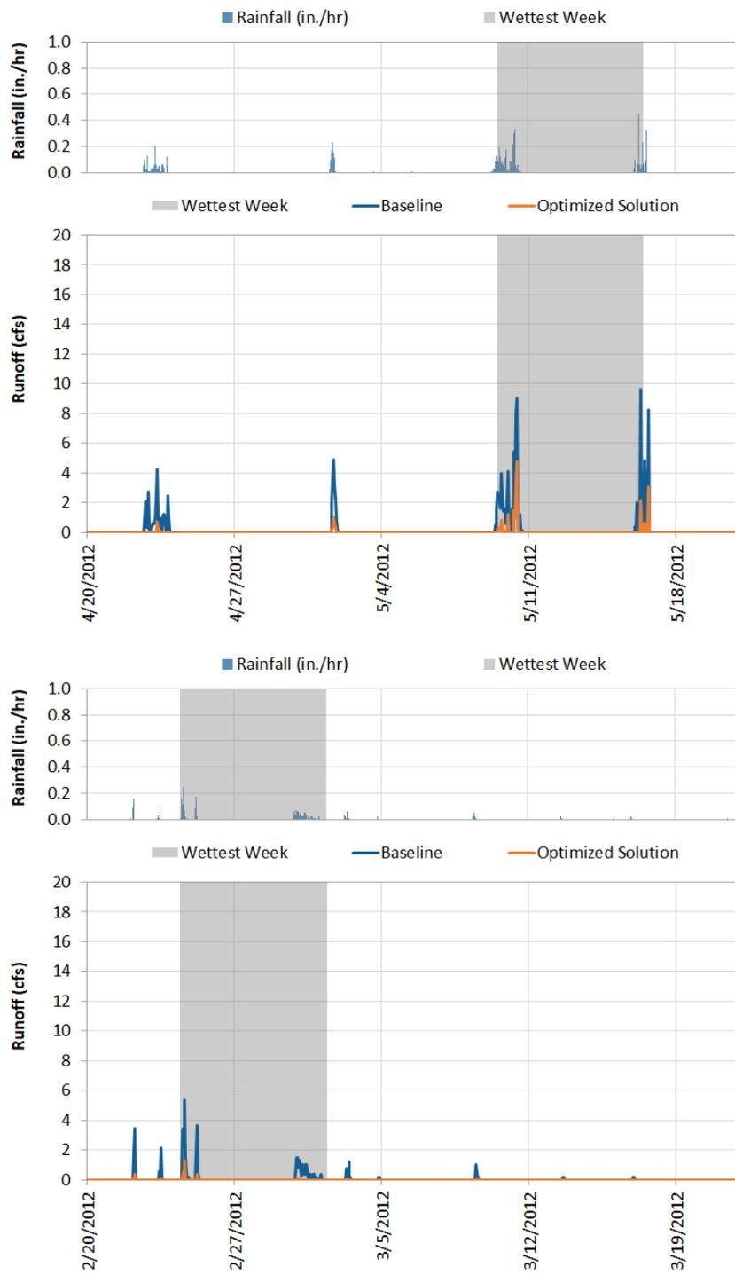
Figure 13. Selected periods of rainfall and runoff for outfall #2 during 2012, a year representing an average amount of precipitation for Tisbury, MA.
