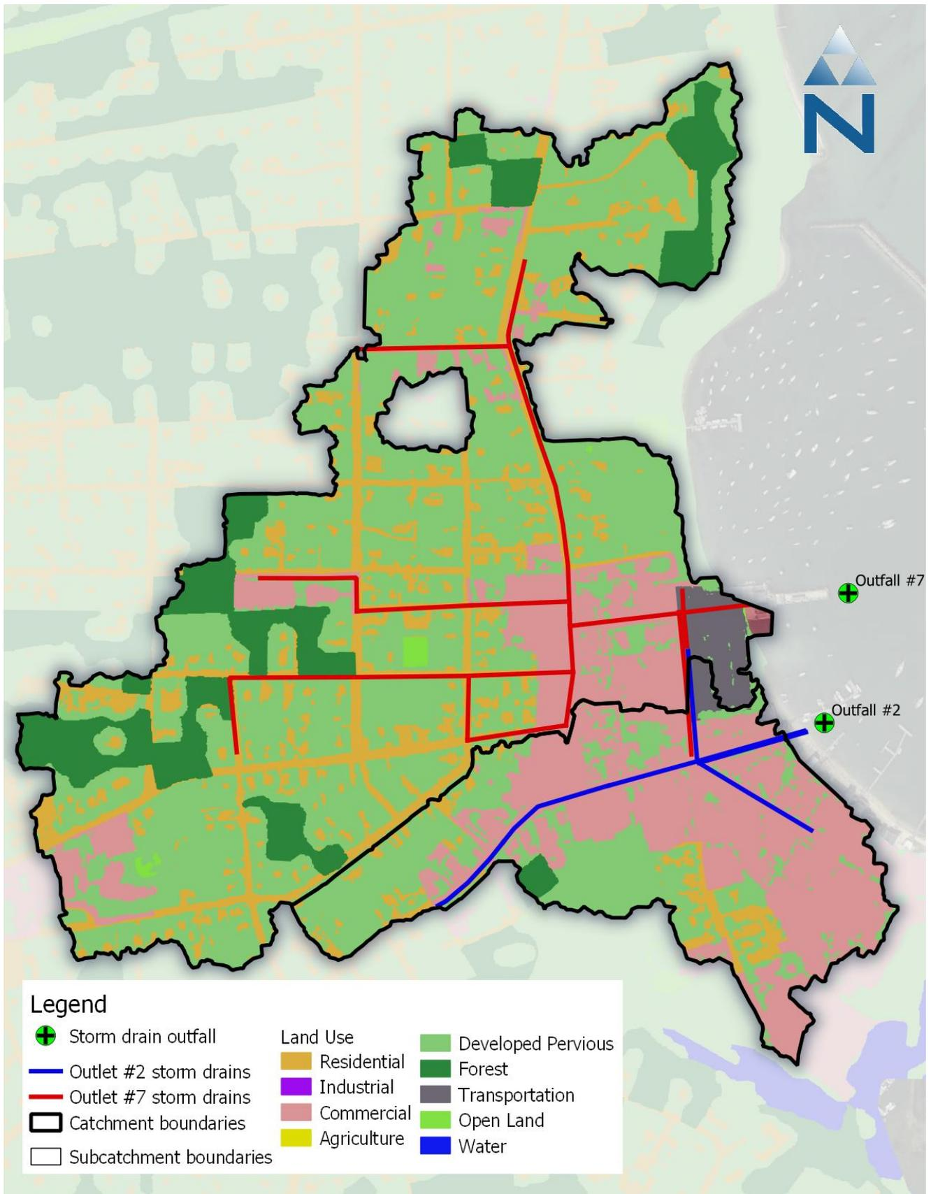
Figure 4. Sub-catchment delineation and major land uses in the drainage areas to outfall #2 and #7.
