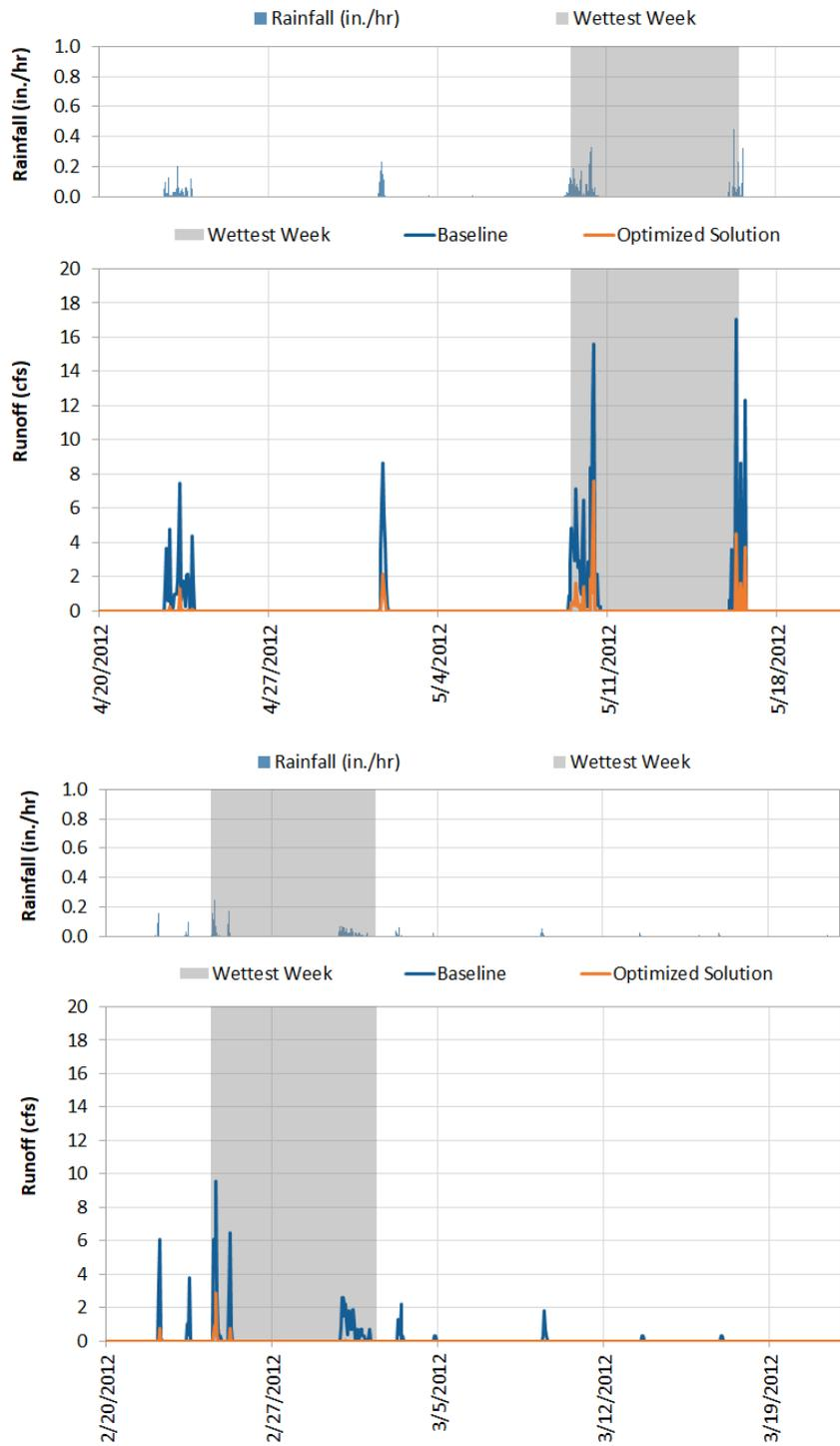
Figure 8. Selected periods of rainfall and runoff for outfall #7 during 2012, a year representing an average amount of precipitation for Tisbury, MA. Grey area highlights the wettest week for the time period shown.
