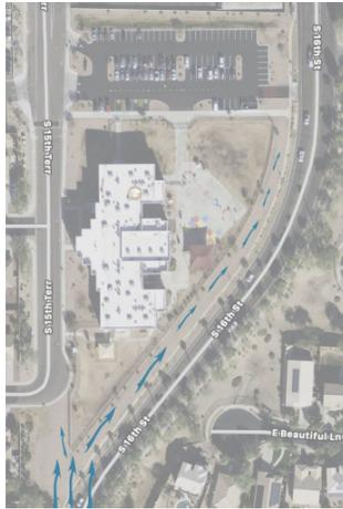
The easement off 16th street includes a bioswale to intercept regional stormwater coming north from South Mountain and prevent it from flooding the schoolyard.
